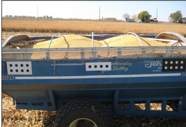
Figure 57: Cart profile with two fill zones
