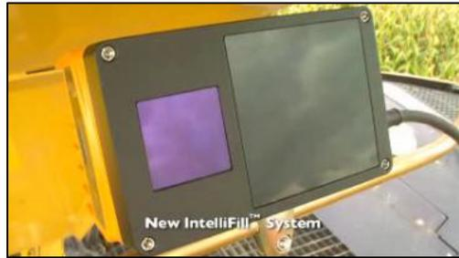
Figure 8: New Holland IntelliFill Time-of-Flight Camera
