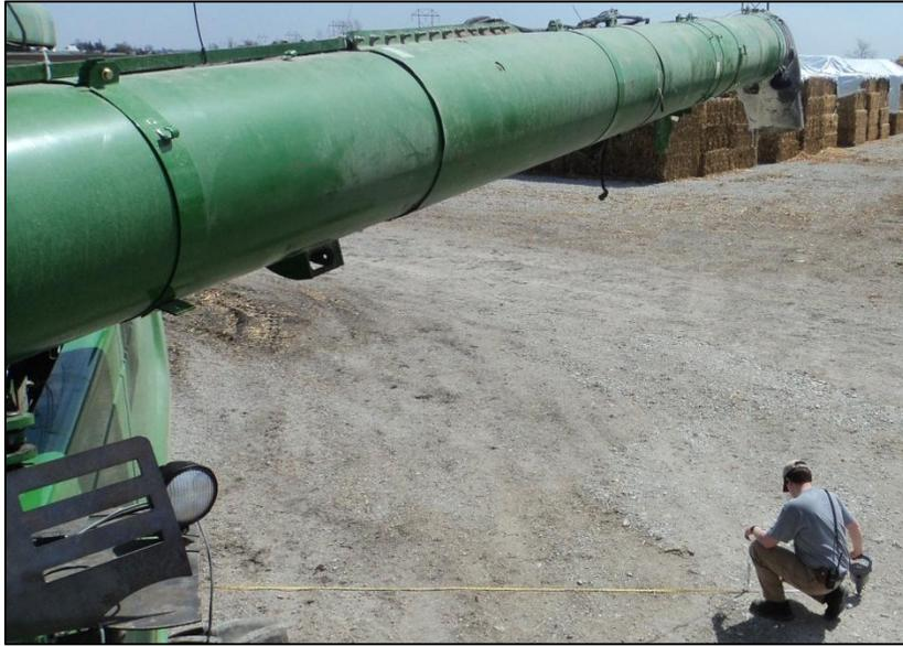
Figure 27: Ground Measurement in Progress for Auger Calibration
