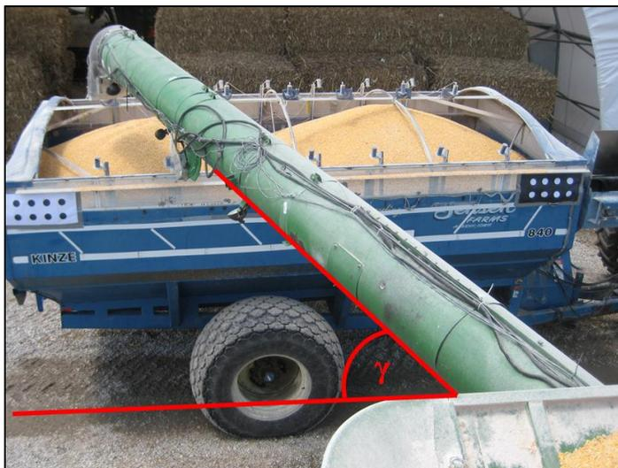
Figure 29: Alternate Auger Angle Depiction
