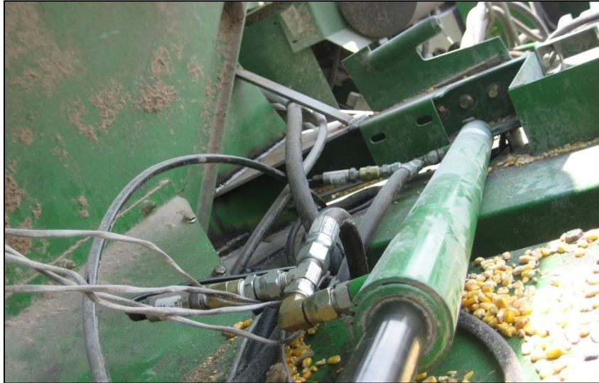
Figure 33: Pressure Sensor Installation
