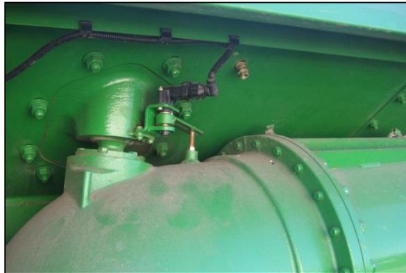
Figure 25: Production Auger-Angle Sensor
