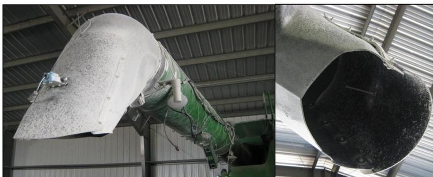
Figure 32: Wobble Sensor Installation
