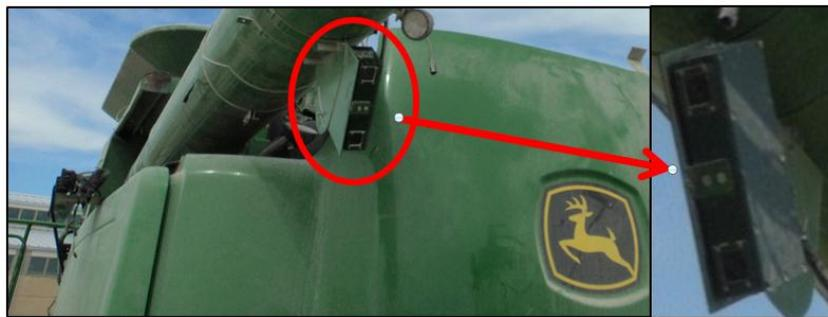
Figure 21: 109 Fill (auger) Camera
