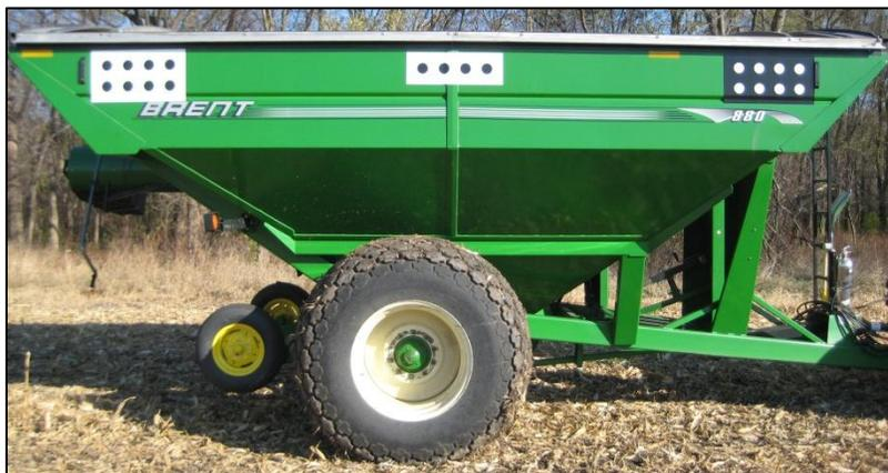
Figure 23: Brent Grain Cart (880bu) with Fiducials
