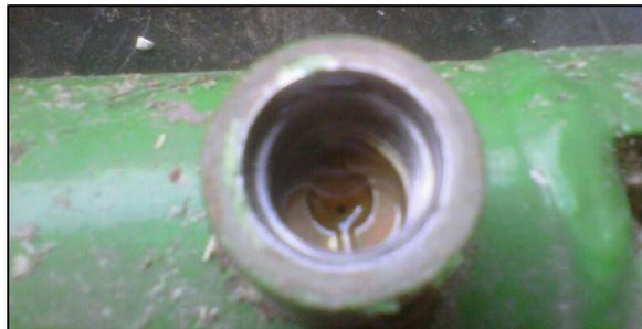
**Figure 16: Orifice in the Cylinder Port**
