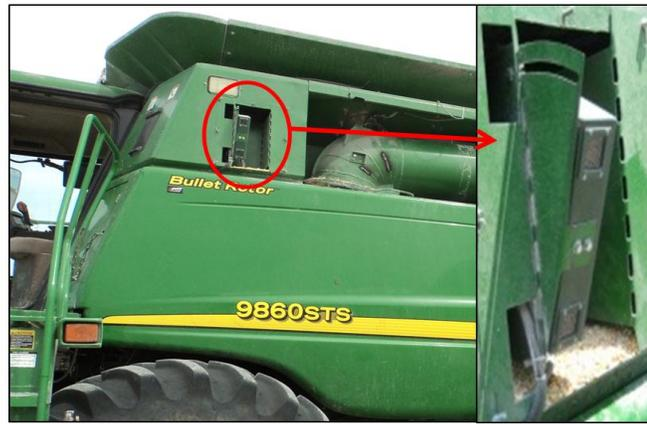
Figure 20: 109 Tracking (grain tank) Camera
