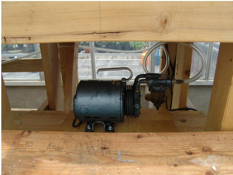
**Figure 5.22** Blower in the Iowa State University tilapia-basil aquaponics (courtesy of Allen Pattillo).
