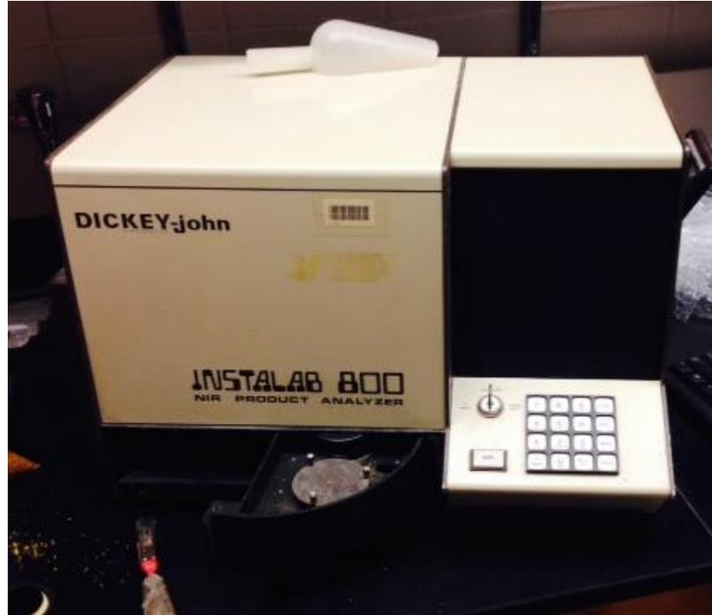
Figure 3.8. DDGS nutrient testing using DICKEY john INSTALAB 800.
