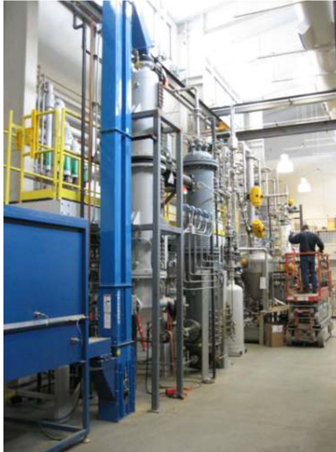
Figure 1: Pilot-scale 20 kg/h fluidized bed gasifier and gas cleaning PDU
