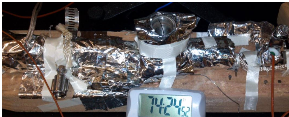
Figure S-4: Heated sampling apparatus for TWA passive sampling at 115°C. Note the thermocouple wire entering the exit side of the glass sampling bulb through a compression T placed in the line (right hand of picture). This thermocouple was routed through the line and placed a few mm from the sampling zone inside the glass bulb. The temperature at this location was used to control the heat tracing for the sample zones (glass bulb and sampling well).
