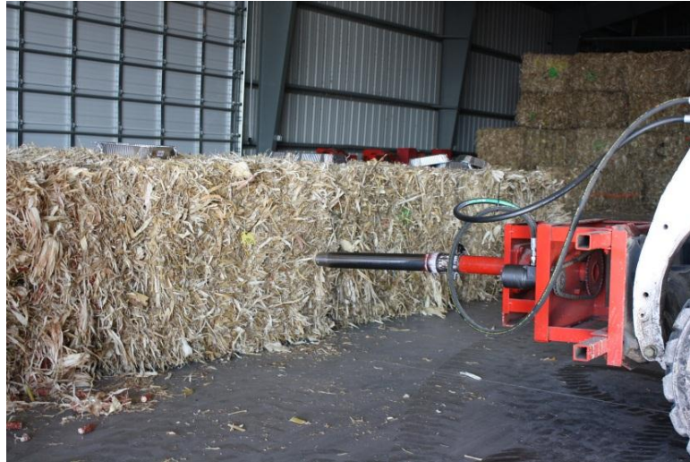
Figure 5.1. Large, 2.5" diameter coring tube attached to the front of a skid loader. The coring tube spins as it drills into the end of a bale to take a sample.
