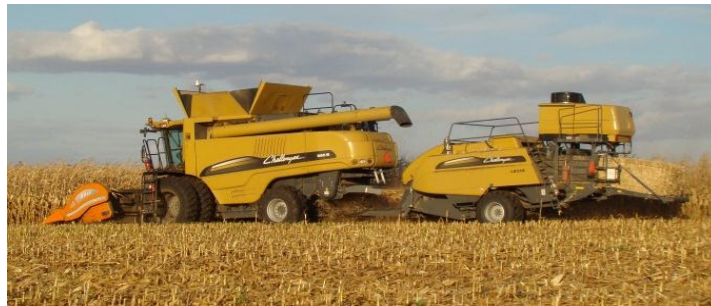
Figure 6.1. AGCO single pass baler producing corn stover bales simultaneously with grain harvest.
