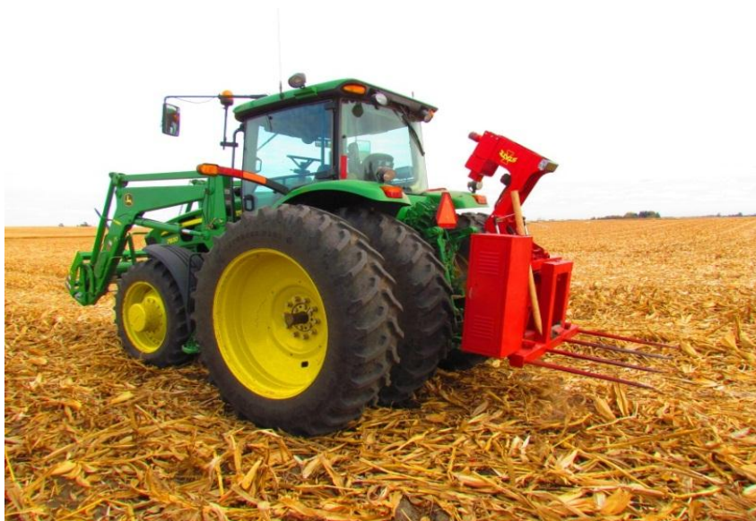
Figure 7.2. Close-up view of the field sampling tool. The forks used to weigh the bale are below, with the coring probe currently up, out of use.
