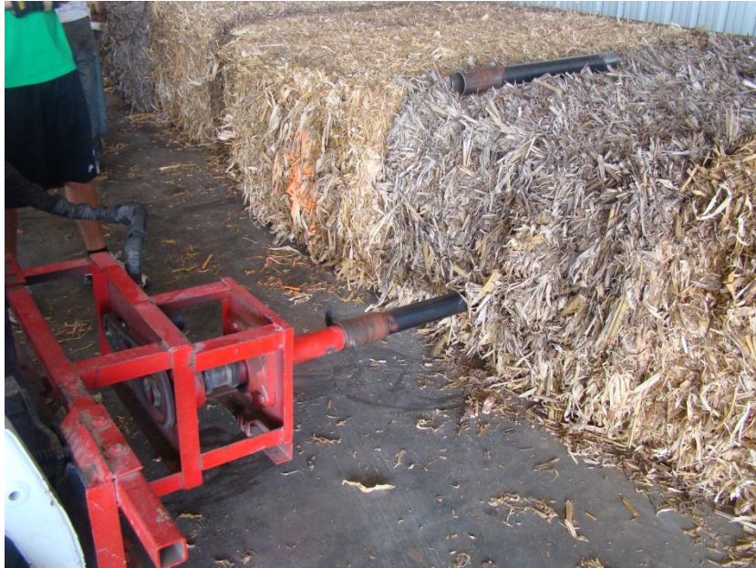
Figure 4.2. The 2.5” core sampler attached to a skid loader taking a core out of a corn stover bale.
