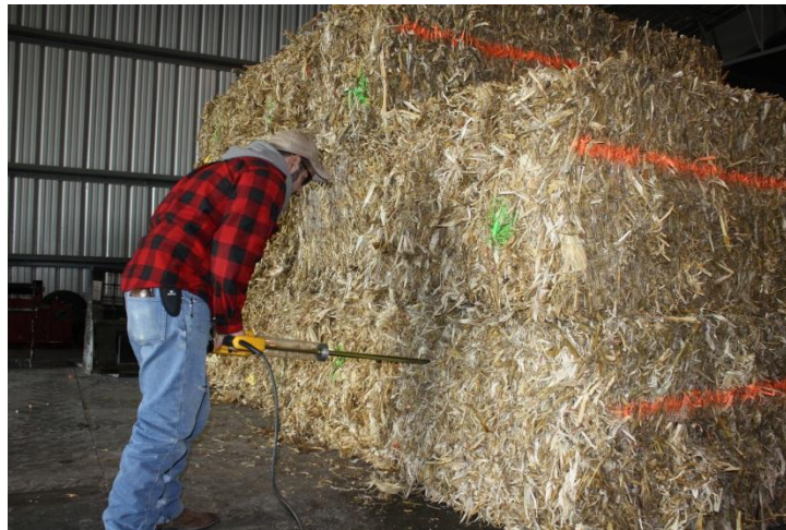
Figure 5.2. Small, \frac{3}{4} " diameter coring tube attached to a portable drill. The coring tube drills into the end of a bale as the operator applies pressure, in order to take a sample.
