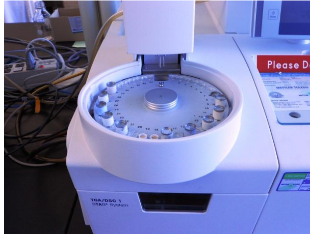
Figure 2.4. Thermogravimetric analyzer used in industrial scale laboratories for material property analysis.
