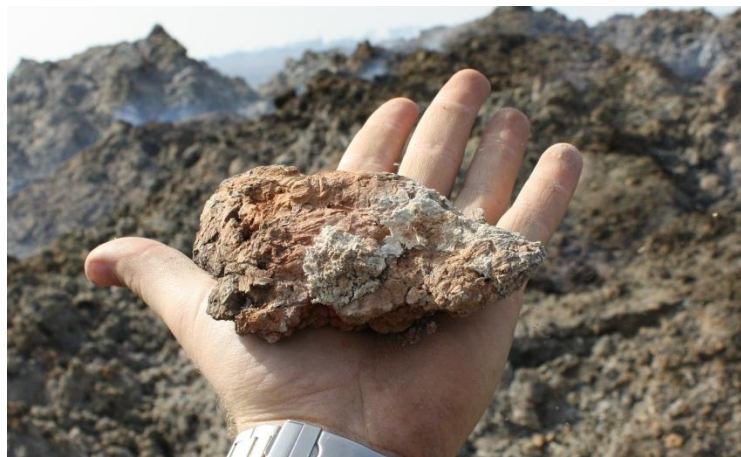
Figure 2.5. Soil remaining after the combustion of a corn stover bale, demonstrating the tendency of the soil to stick together when in the presence of high temperatures.
