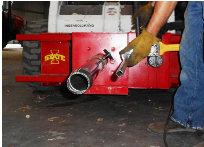
Figure 5.3. Two different sizes of sampling tools were used, a large, 2.5" diameter coring tube (left) and a small, 3/4" coring tube (right). The ends of both tools have boring teeth.
