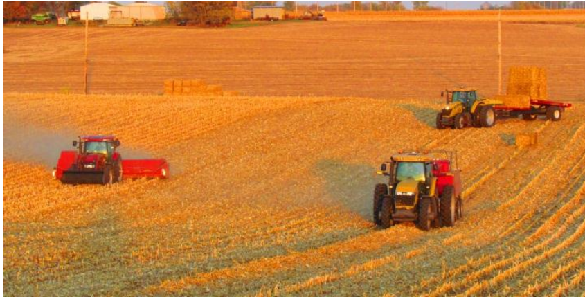
Figure 6.2. Multipass harvesting, shredder windrower on the far left, baler making bales from a windrow on the right front, and a bale stacker behind.
