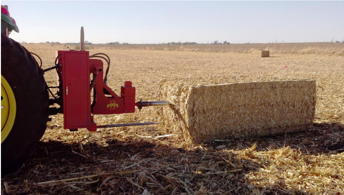
Figure 7.1. Field sampling tool in the process of sampling a bale.
