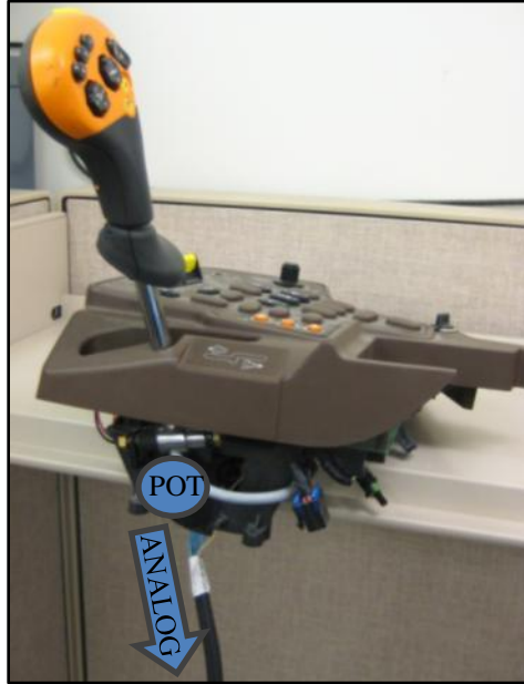
Figure 4.1: Hydro Handle setup for propel-by-wire
