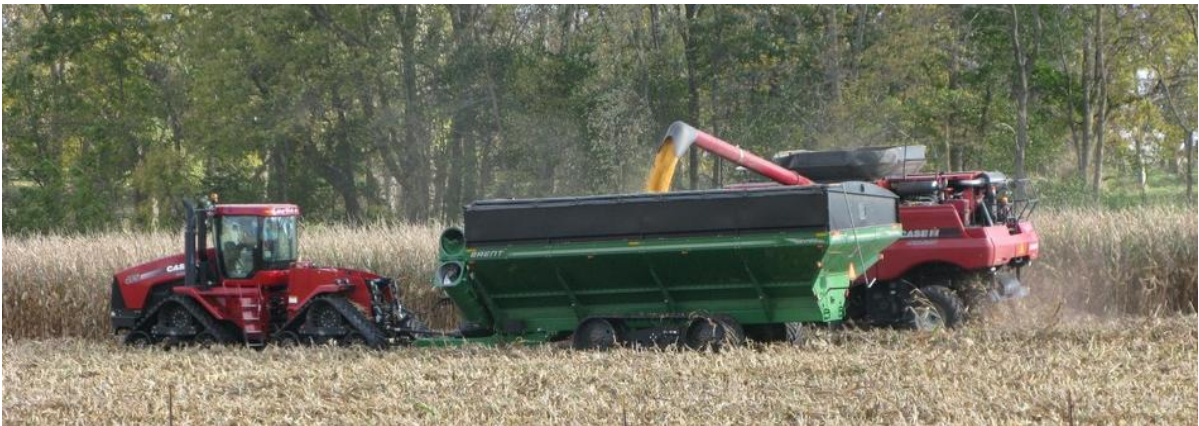
Figure 4.2: Brent 2000 bu. grain cart with a fillable length of 9.75 m (Photo credit: The Mitchell Farm)
