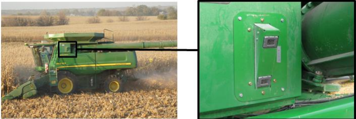
Figure 4.7: Tracking camera mounted on the side of the combine.
