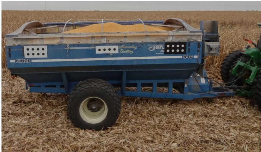
Figure 4.8: Grain cart with three targets installed for tracking
