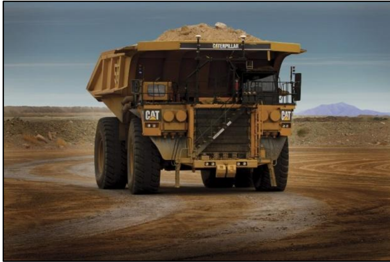
Figure 2.3 A Cat Mining Truck using Minestar software and GNSS position information to operator autonomously. (Photo credit: Caterpillar)
