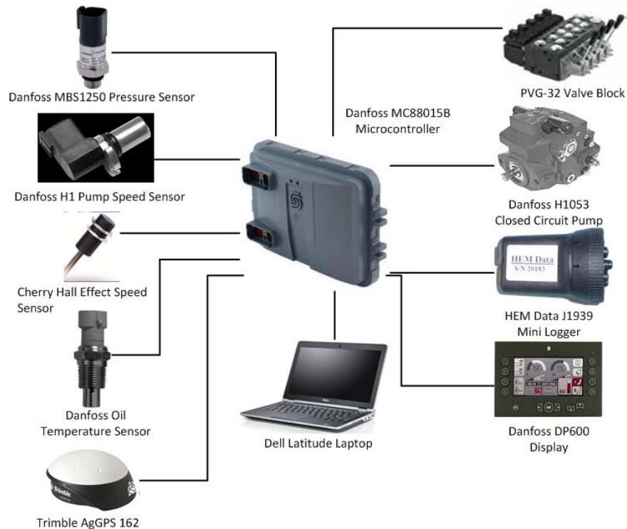
Figure 8.1: Simplified Harvester Electrical Schematic
