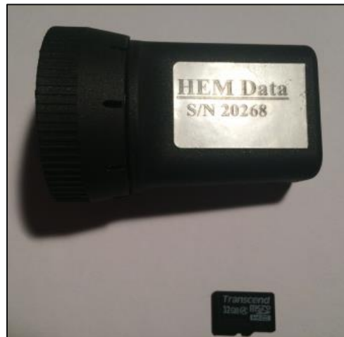
Figure 8.9: HEM Data J1939 Mini Logger for Logging CAN Messages via the ISO Bus Port
