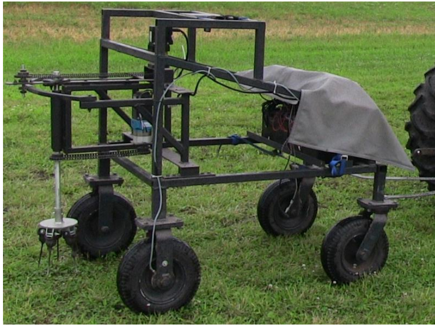
Figure 3.13: Fabricated prototype of the weed actuation system.
