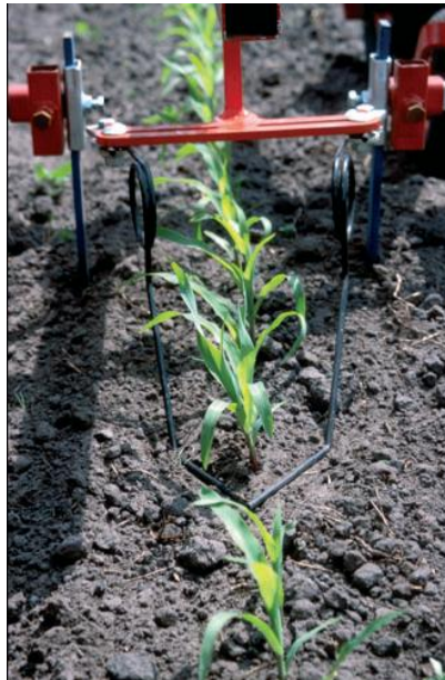
Figure 2.4: Torsion weeder uses flexible coil spring tines to sweep the weeds ( Weide et al., 2008).
