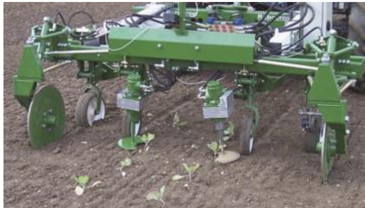
Figure 2.9: Automated weeder machine using hydraulics to rotate semi-circle discs that are used for weed control (Tillett et al., 2008).
