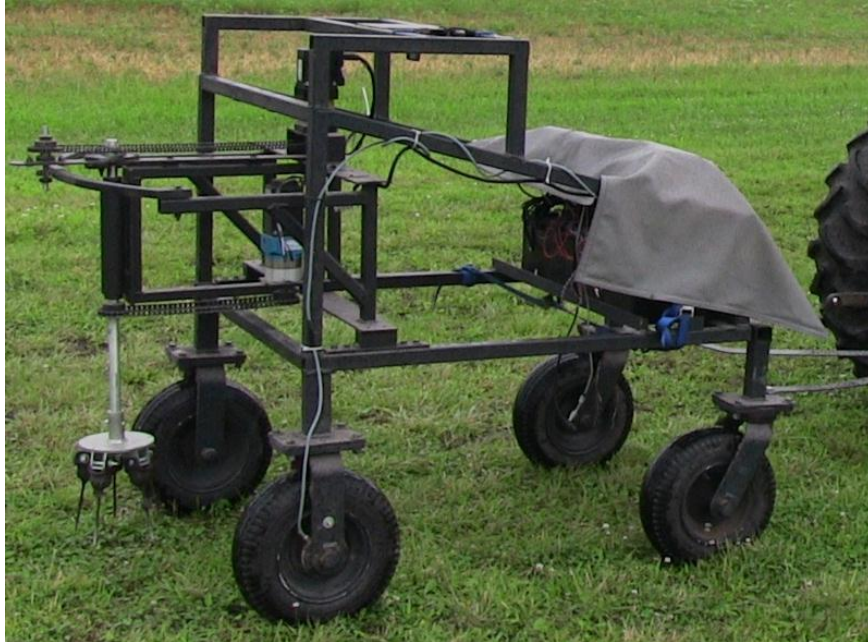
Figure 4.2: Rotating tine mechanism consisted of a disc with tines mounted on it. The mechanism is driven by a BLDC motor using a chain drive system.
