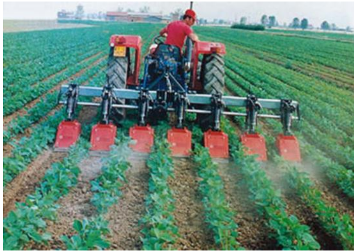
Figure 2.1: Inter-row rotary cultivator for inter-row weed control (Tornado, 2011).
