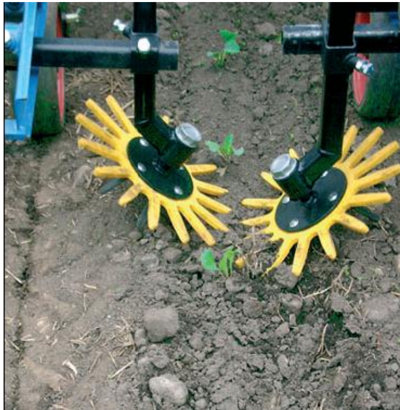
Figure 2.3: Finger weeder uses rubber spikes that are pointed at an angle towards the crop ( Weide et al., 2008).
