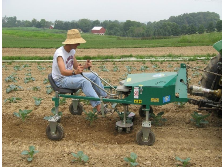
Figure 2.6: ECO weeder uses rotating weeding mechanisms with tines (Hillside Cultivator Company, 2011).
