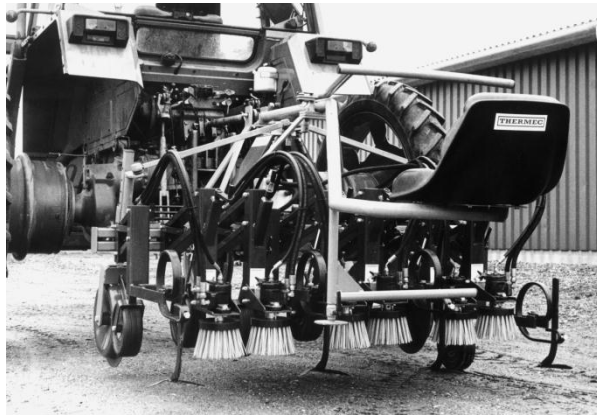
Figure 2.5: Vertical-rotating brush weeder use hydraulics and require an operator to control the brushes (Melander, 1997).
