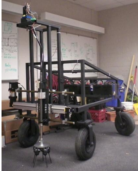
Figure 3.9: Fabricated prototype developed positioned the weeding mechanism motor on a vertical position which made it difficult when the actuation system was moving sideways.
