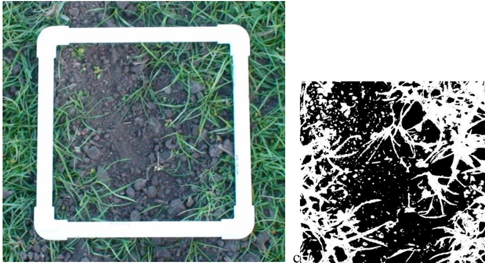
Figure 4.4: Left image shows the machine weeding inside a quadrat frame. Right image shows the processed image used for calculating weed pixel reduction.
