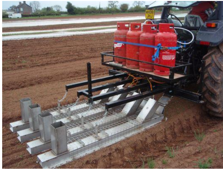
Figure 2.7: A crop-row flame weeder using LPG gas to control weeds inside the crop row (Physical Weeding, 2011).
