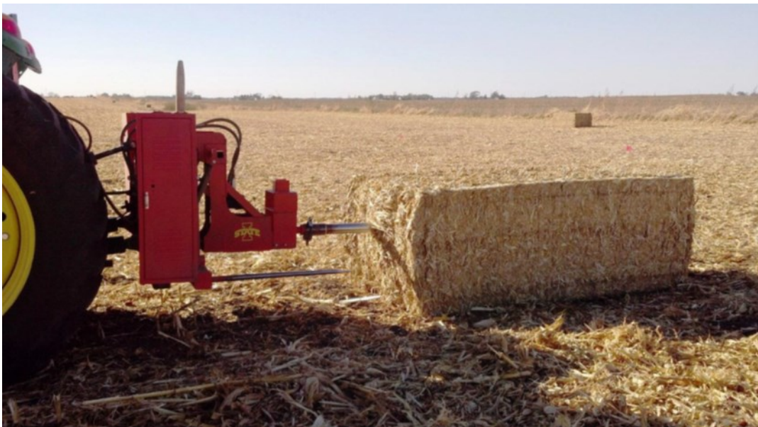
Figure 1: Large square bale sampler with the 2.5-inch diameter coring probe drilling into the end of the corn stover bale
