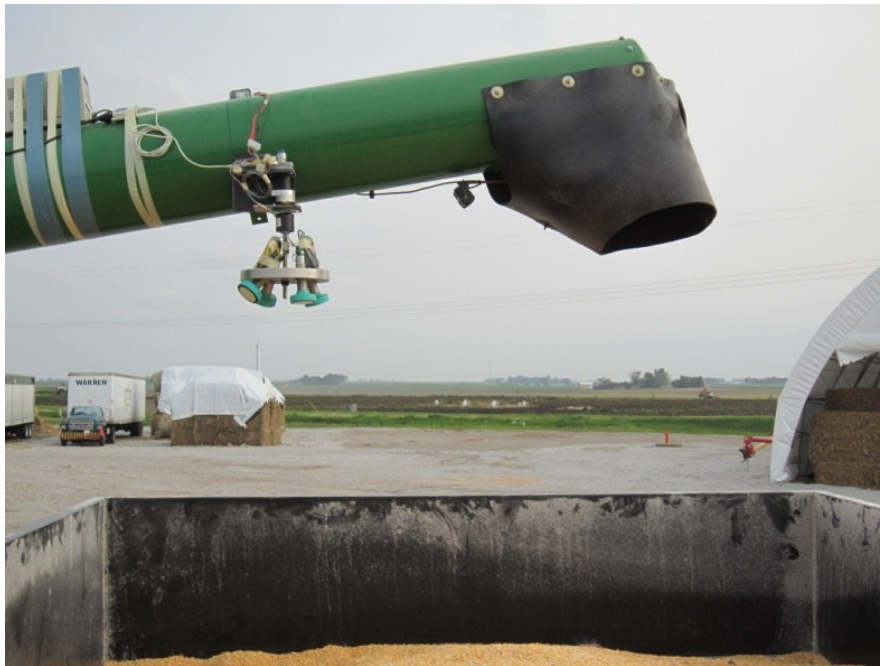
Figure 4. Sensor package mounted on combine harvester unloading auger.
