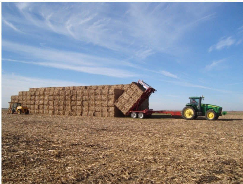
Figure 10: Morris Industries 16K Plus Bale Runner adding bales to a stack
