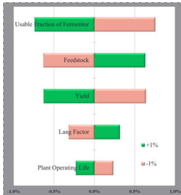
Figure 1: Top five sensitivity coefficients using a \pm 1\% change in BioPET model under expected values for bioproduction of styrene (x-axis represents measured change in MESP).
