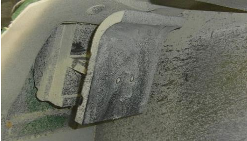
Figure 2.2: Current impact plate model installed on a John Deere combine at the BioCentury Research Farm
