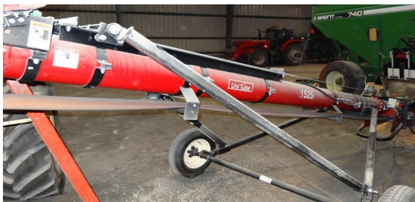
Figure 4.5: Belt conveyor selected as the method of grain delivery
