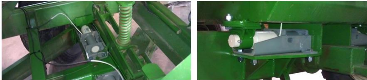
Figure 4.3: Ground truth measurement system installed on the test stand wagon, (left) load cell mounted on the front half of the wagon frame, (right) load cell mounted on the back of the wagon frame
