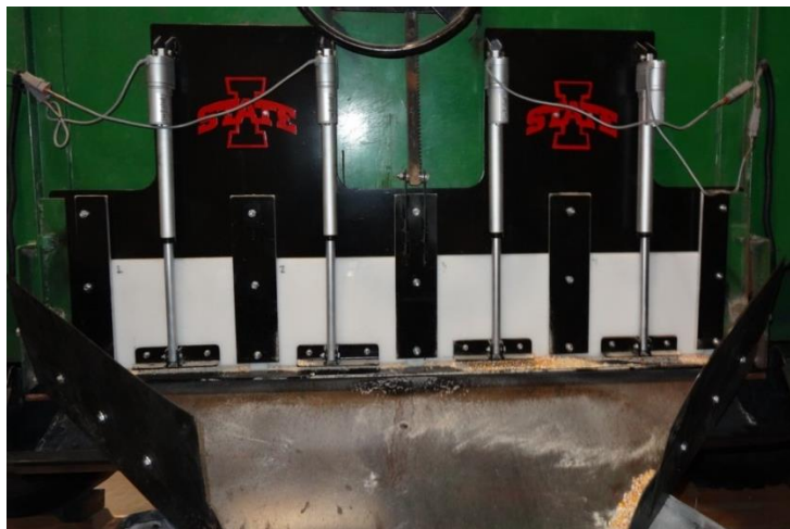
Figure 4.2: Customized wagon gate developed for metering grain into the test stand
