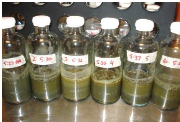
Figure 2. A set of samples after seven days of incubation for the methane production rate assay.
