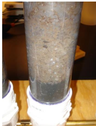
Figure 1. A lab-scale illustration of a three-phase foam (AWML, Iowa State University).
