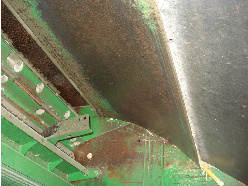
Figure 14: Image of impact plate taken after Fall 2011 harvest showing wear patterns in paint caused by impacting stover.
