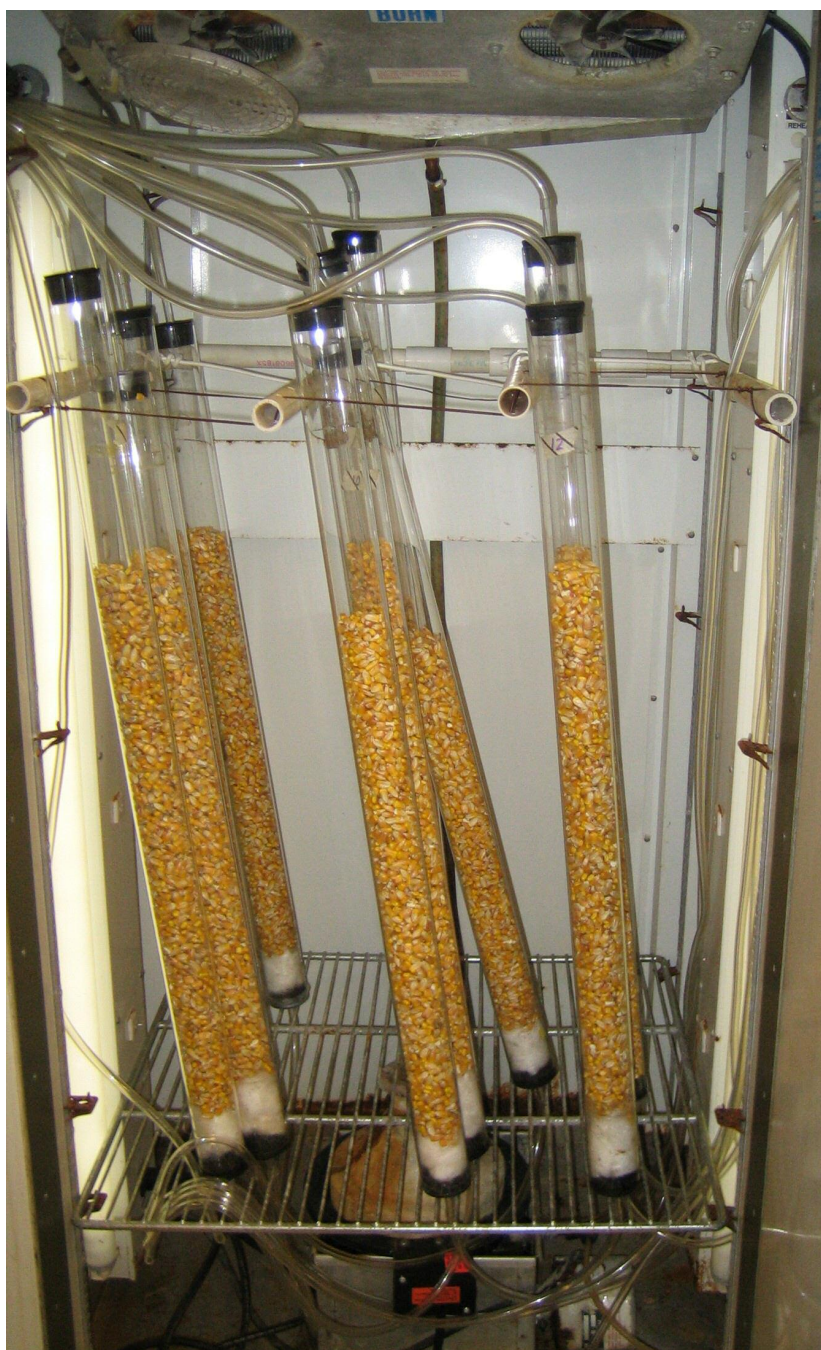
Figure 2.2 Environmental chamber with grain storage units (environmental chamber lights on only for purpose of picture)
