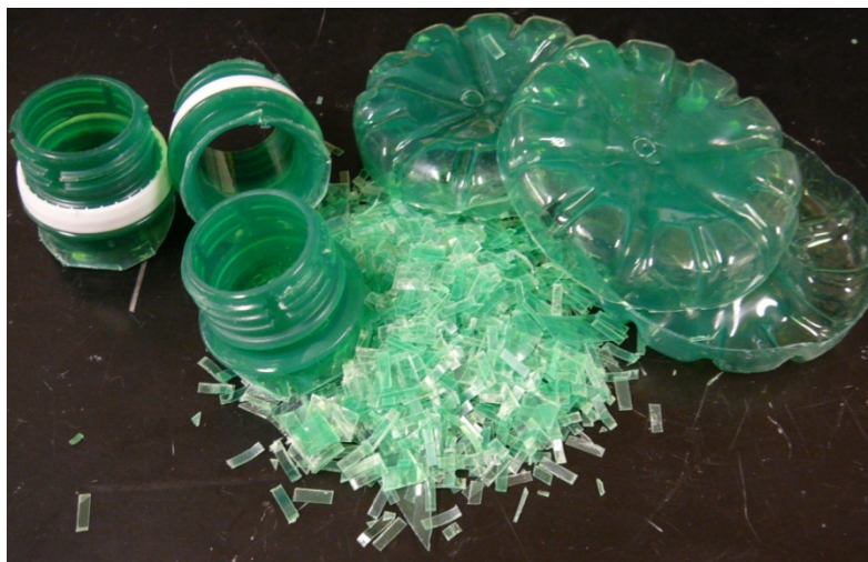
Figure 28 Chopped PLA chips from postconsumer water bottles (Picture showing unused neck and bottom portions)
