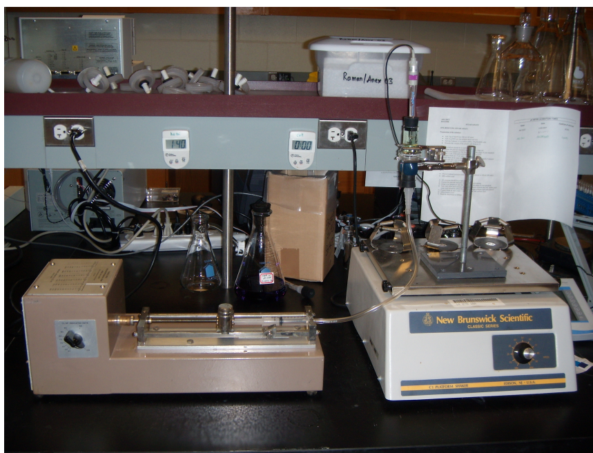
Figure 3.2: Photograph of testing apparatus for pH-color indicator solution
