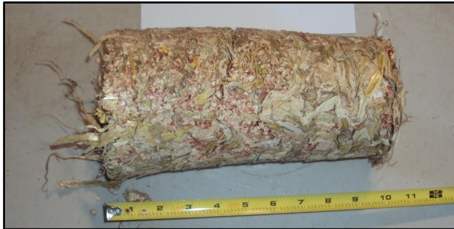
Figure 7.6. Briquette produced during the material types experiment. (14 MPa compression pressure, 11%MCwb, MOG)
