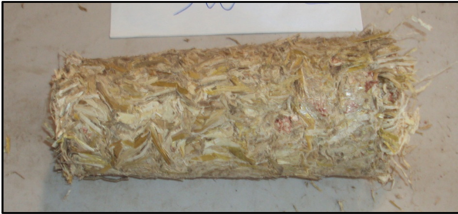
Figure 5.10. Briquette produced during the 3-way interaction experiment. (14 MPa compression pressure, 8.3% MCwb, 42 mm particle size)
