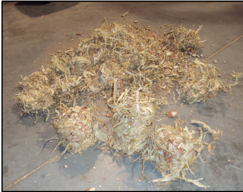
Figure 9.9. Output product from an 'as received' MOG tumbler test
