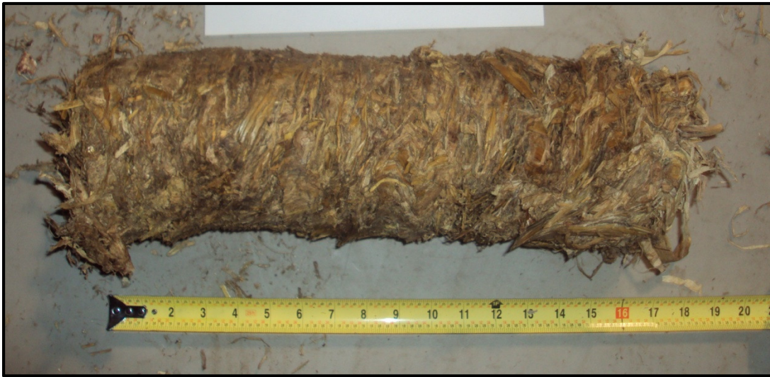
Figure 6.8. Briquette produced during the moisture effects experiment. (14 MPa compression pressure, 24.8% MCwb, 3.6° die taper angle)
