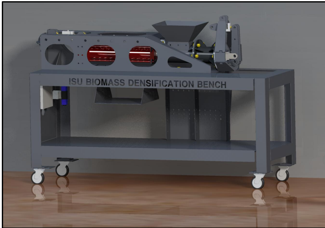
Figure 3.1. CAD model of the densification test bench
