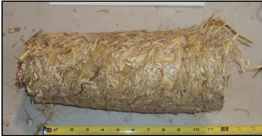
Figure 5.11. Briquette produced during the 3-way interaction experiment. (14 MPa compression pressure, 8.3% MCwb, 42 mm particle size)
