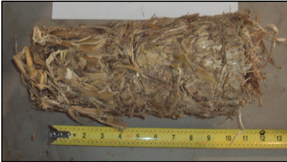
Figure 6.11. Briquette produced during the moisture effects experiment. (9 MPa compression pressure, 13.0% MCwb, 7.2° die taper angle)
