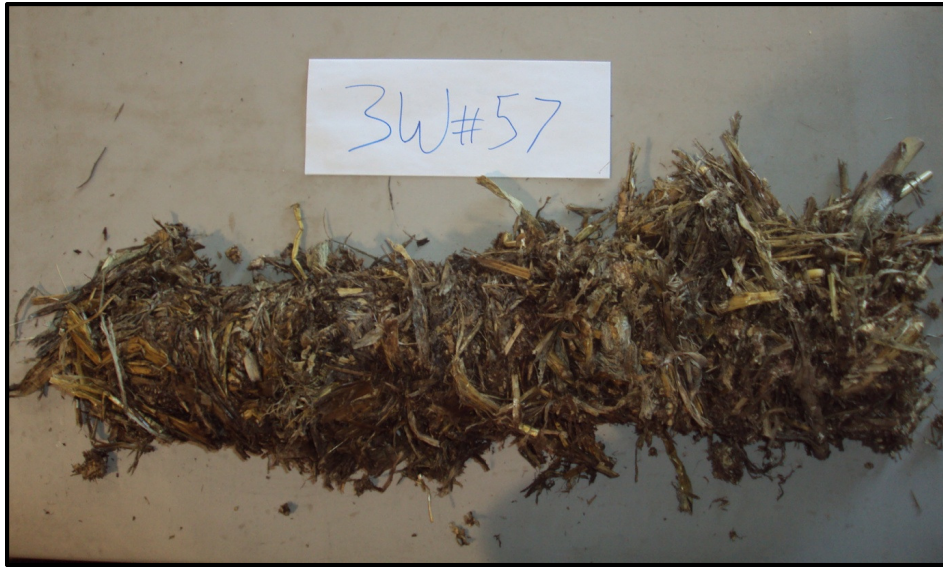
Figure 9.5. Briquette produced at 54.5% moisture content.
