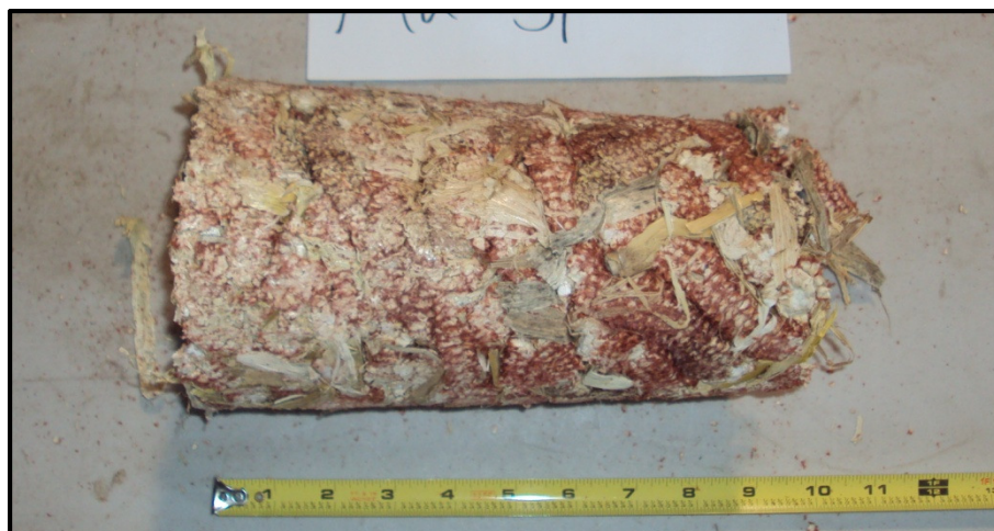
Figure 7.7. Briquette produced during the material types experiment. (14 MPa compression pressure, 10% MCwb, pure cobs)
