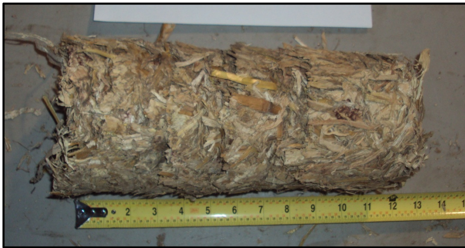
Figure 6.10. Briquette produced during the moisture effects experiment. (9 MPa compression pressure, 13.0% MCwb, 3.6° die taper angle)
