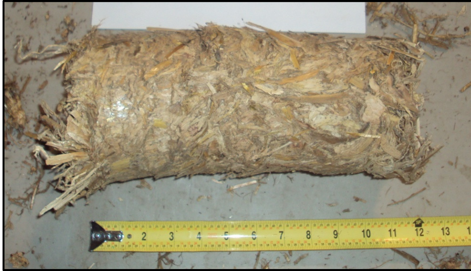
Figure 6.7. Briquette produced during the moisture effects experiment. (14 MPa compression pressure, 13.0% MCwb, 3.6° die taper angle)
