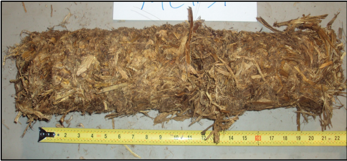
Figure 6.9. Briquette produced during the moisture effects experiment. (14 MPa compression pressure, 47.6% MCwb, 3.6° die taper angle)
