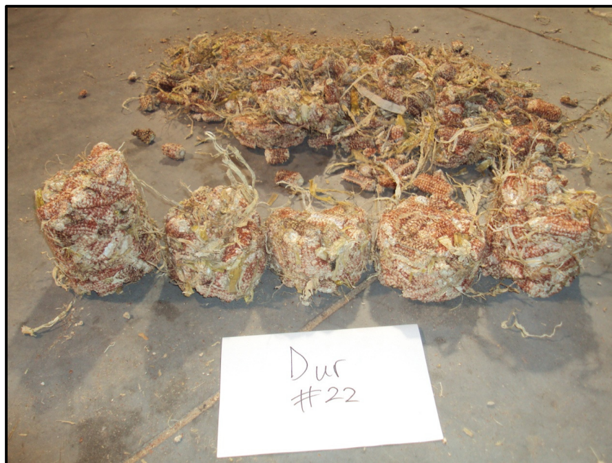
Figure 9.10. Output product from an 'as received' pure cob tumbler test
