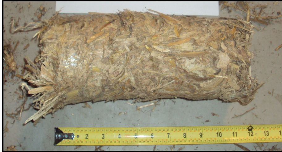
Figure 7.5. Briquette produced during the material types experiment. (14 MPa compression pressure, 13%MCwb, corn stover)
