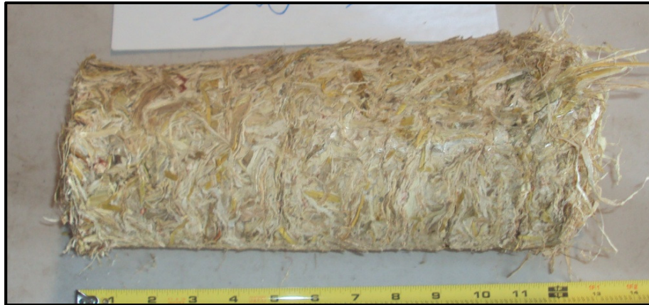
Figure 5.12. Briquette produced during the 3-way interaction experiment. (14 MPa compression pressure, 8.3% MCwb, 22 mm particle size)
