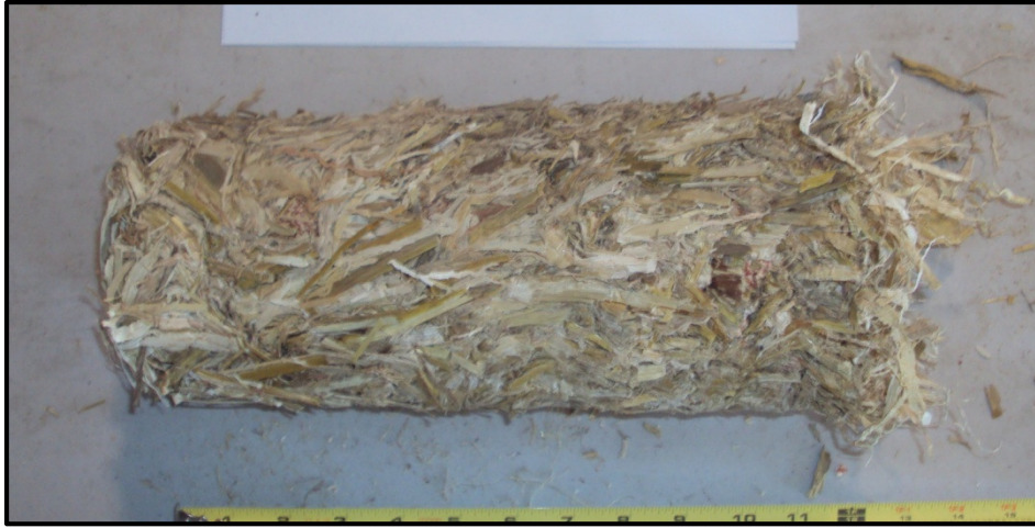
Figure 5.9. Briquette produced during the 3-way interaction experiment. (7 MPa compression pressure, 8.3% MCwb, 42 mm particle size)
