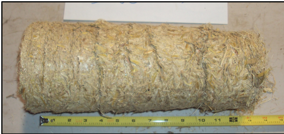
Figure 5.13. Briquette produced during the 3-way interaction experiment. (14 MPa compression pressure, 8.3% MCwb, 19 mm particle size)
