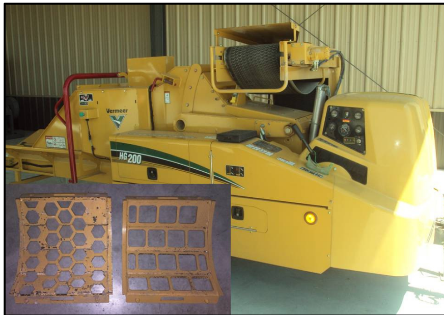
Figure 3.12. Vermeer HG200 grinder and screens
