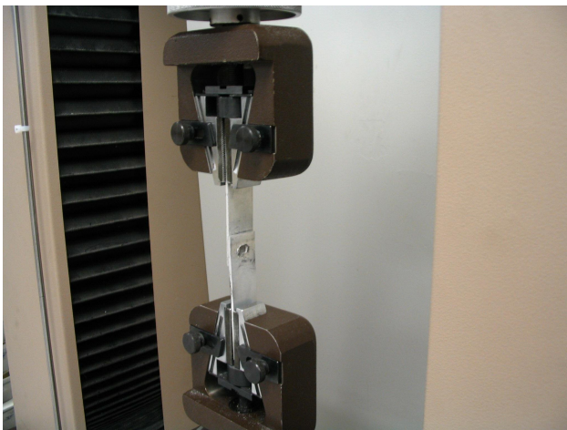
Figure 17 Picture of the testing equipment while measuring the weld strength
