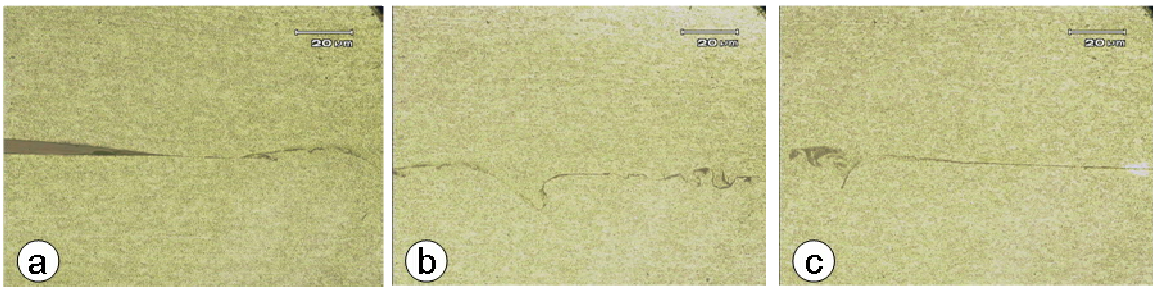
Figure 64 50X micrographs of the welding area of the sample welded with a postheight of 4.75 mm (a) left edge of weld (b) center of weld and (c) right edge of weld
