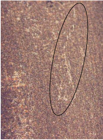
Figure 44 Optical micrograph of the weld area of the sample without copper sheet at 5X
