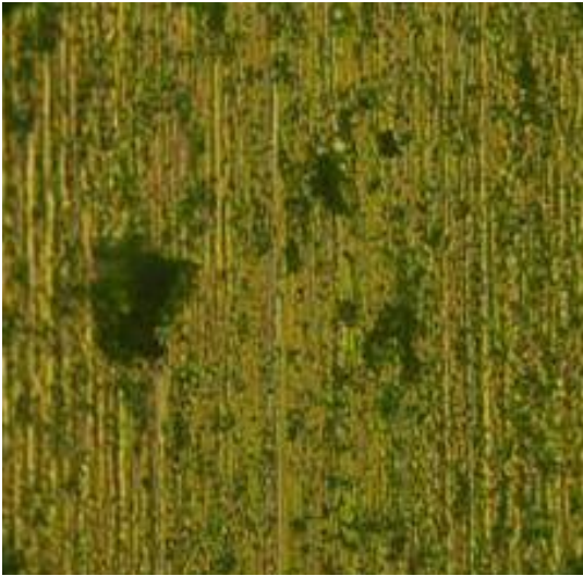
Figure 45 Optical micrograph of the welding area of the sample without copper sheet at 100X
