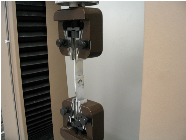
Figure 59 Picture of the testing weld strength
