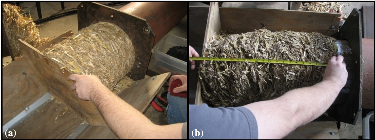
Figure 10. Using a piece of plywood to ensure an accurate ejected length
