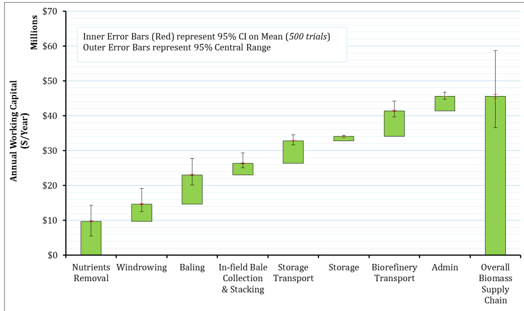
Figure S2.1: Annual working capitals for different processes of the corn stover biomass supply chain of a 114 MLPY (30 MGPY) biorefinery plant
