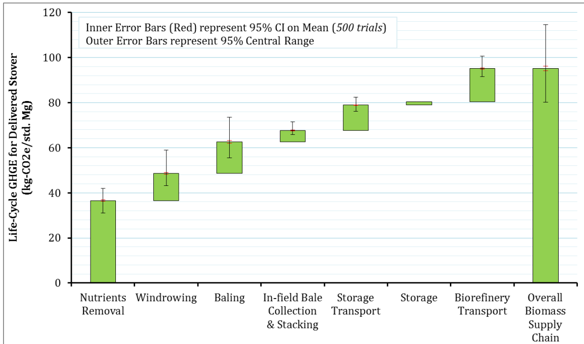
Figure 3.2: Life-cycle GHGE for delivering corn stover biomass feedstock to the gate of a Midwest-based 114 MLPY (30 MGPY) cellulosic biorefinery
