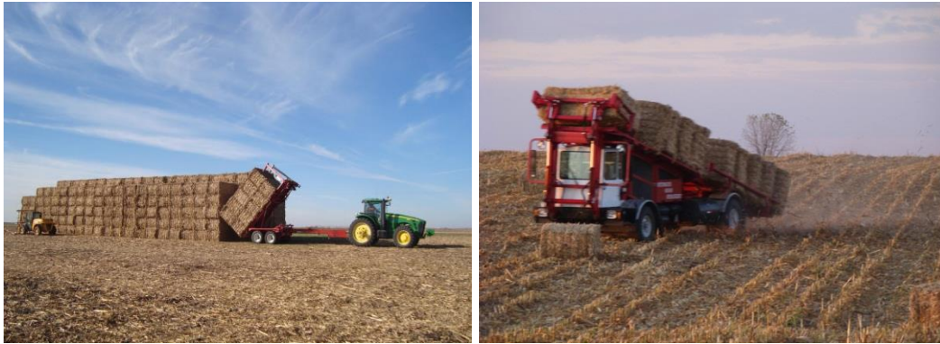
Figure 1.7: In-field multi-bale collection wagon in action (Left picture shows the externally-powered pull-type multi-bale collection wagon; and right picture shows the self-propelled Stinger multi-bale collection wagon) (Note: left picture modified from Darr and Shah (2012) )
