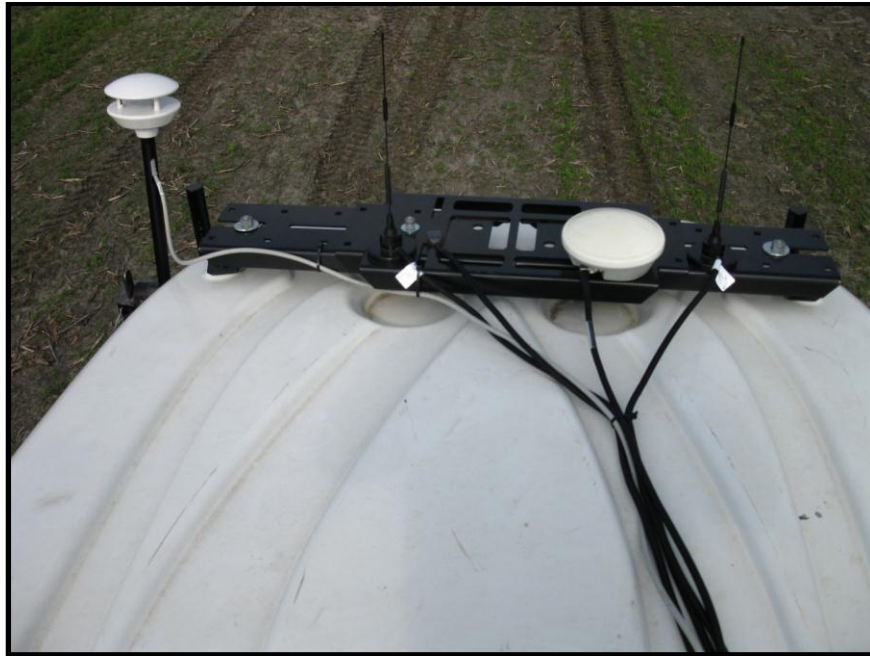
Figure 40. Weather station, RTK cellular and GPS antennas
