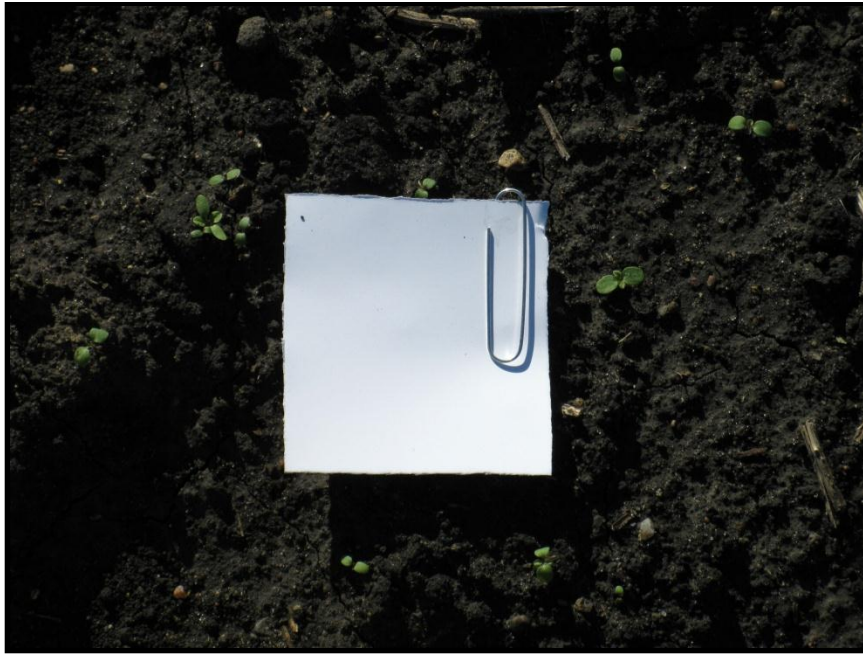
Figure 47. Kromekote collection card with paperclip fixture
