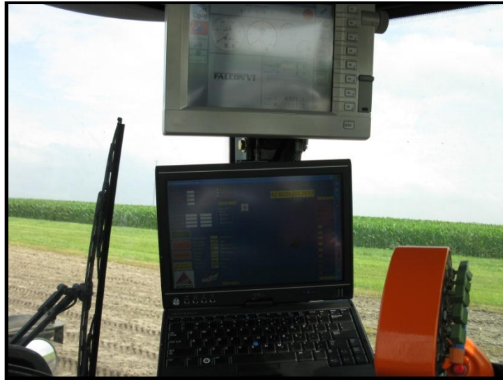
Figure 39. Laptop mounted in cab under rate controller
