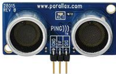
Figure 31. Ping))) ultrasonic sensor (Parallax Inc.) instrumented to measure boom height
