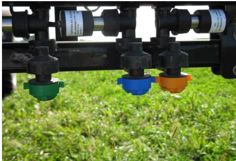
Figure 26. Very coarse, coarse, and fine nozzle bodies with activating solenoids on test machine
