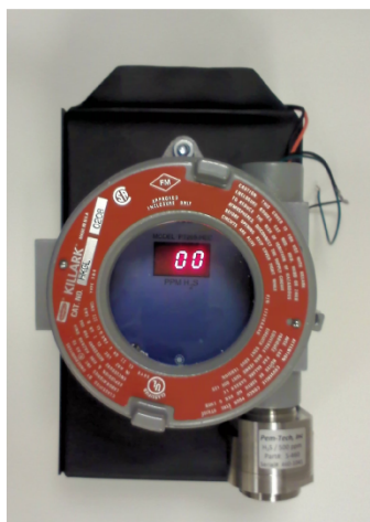
Figure 4.2. Hydrogen sulfide wireless sensor units measured high concentration hydrogen sulfide within the swine barn during manure removal and agitation events.
