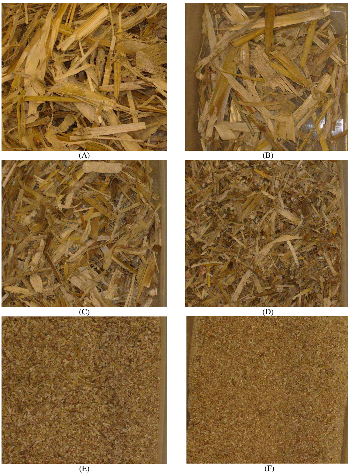
Figure A5. Photographs of stover material after particle reduction with a roller mill at a nominal feedrate of 126 kg/hr and roller gap setting of 0.0889 cm. Material collected over 5.08 cm screen (A), 2.54 cm screen (B), 1.27 cm screen (C), 0.635 cm screen (D), 0.318 cm screen (E) and above pan (F), are shown.
