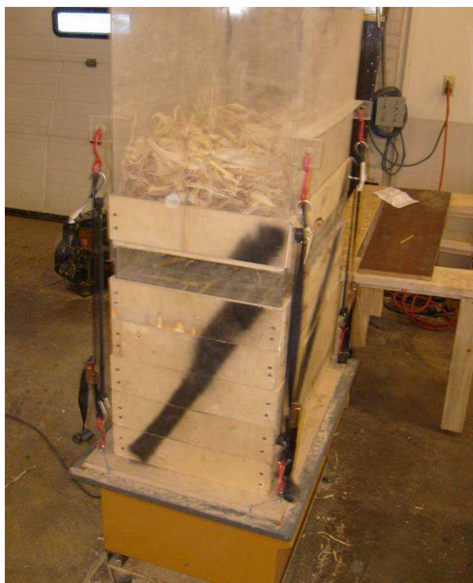
Figure 7. Shaker and screen used to sift material.
