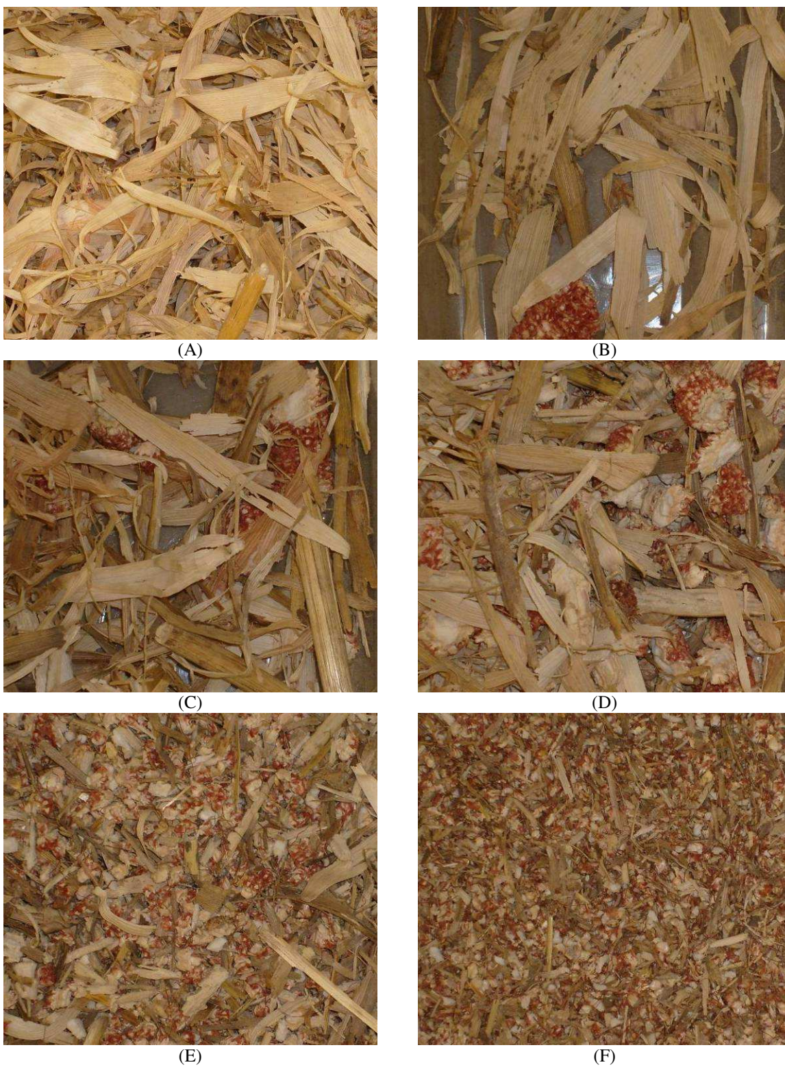
Figure B3. Photographs of raw stover material collected from rear of combine with conventional corn head and standard flail type chopper. Material collected over 7.62 cm screen (A), 5.08 cm screen (B), 2.54 cm screen (C), 1.27 cm screen (D), 0.635 cm screen (E) and above pan (F), are shown.
