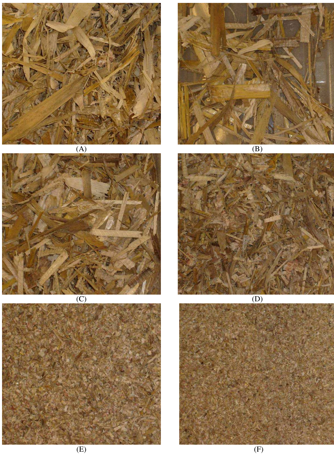
Figure A3. Photographs of stover material after particle reduction with a roller mill at a nominal feedrate of 126 kg/hr and roller gap setting of 0.0254 cm. Material collected over 5.08 cm screen (A), 2.54 cm screen (B), 1.27 cm screen (C), 0.635 cm screen (D), 0.318 cm screen (E) and above pan (F), are shown.
