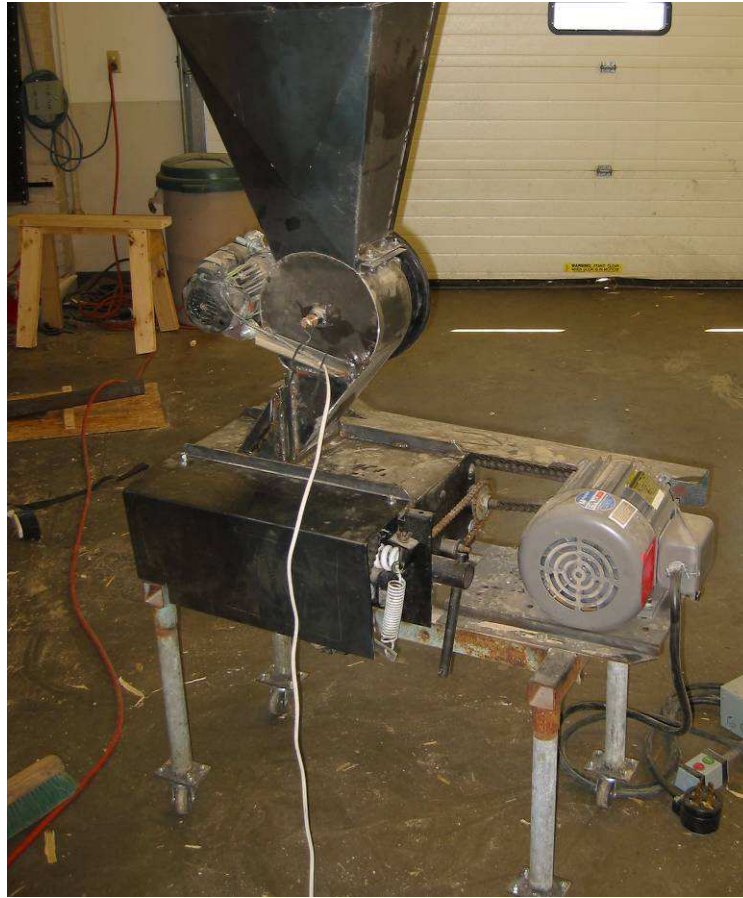
Figure 6. Rollermill assembled with feed unit.
