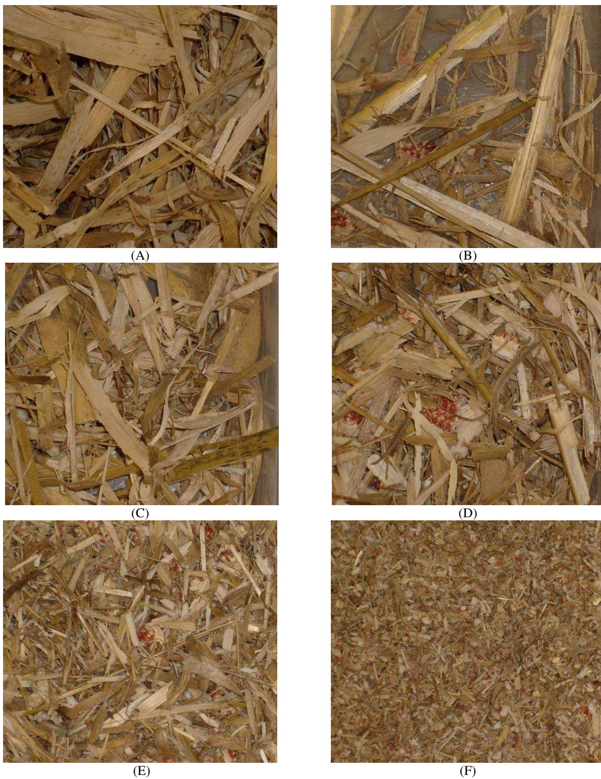
Figure B4. Photographs of raw stover material collected from rear of combine with row crop head and standard flail type chopper. Material collected over 7.62 cm screen (A), 5.08 cm screen (B), 2.54 cm screen (C), 1.27 cm screen (D), 0.635 cm screen (E) and above pan (F), are shown.
