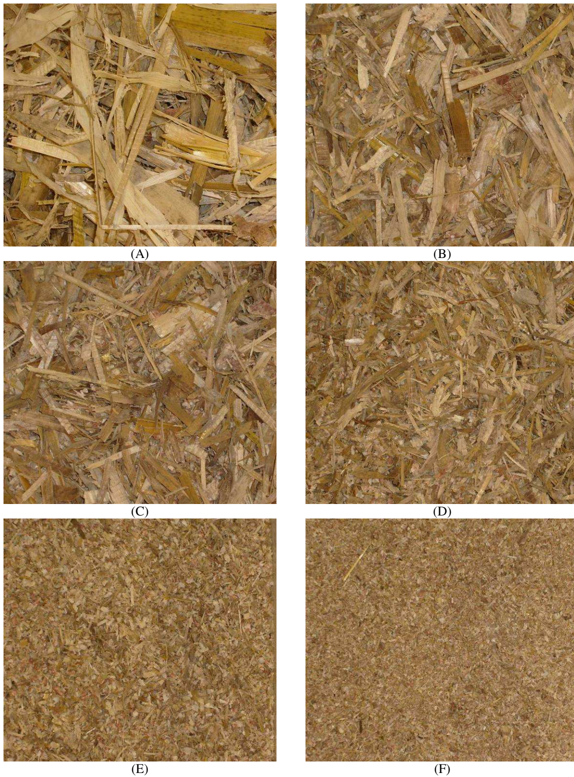
Figure A2. Photographs of stover material after particle reduction with a roller mill at a nominal feedrate of 84 kg/hr and roller gap setting of 0.0254 cm. Material collected over 5.08 cm screen (A), 2.54 cm screen (B), 1.27 cm screen (C), 0.635 cm screen (D), 0.318 cm screen (E) and above pan (F), are shown.
