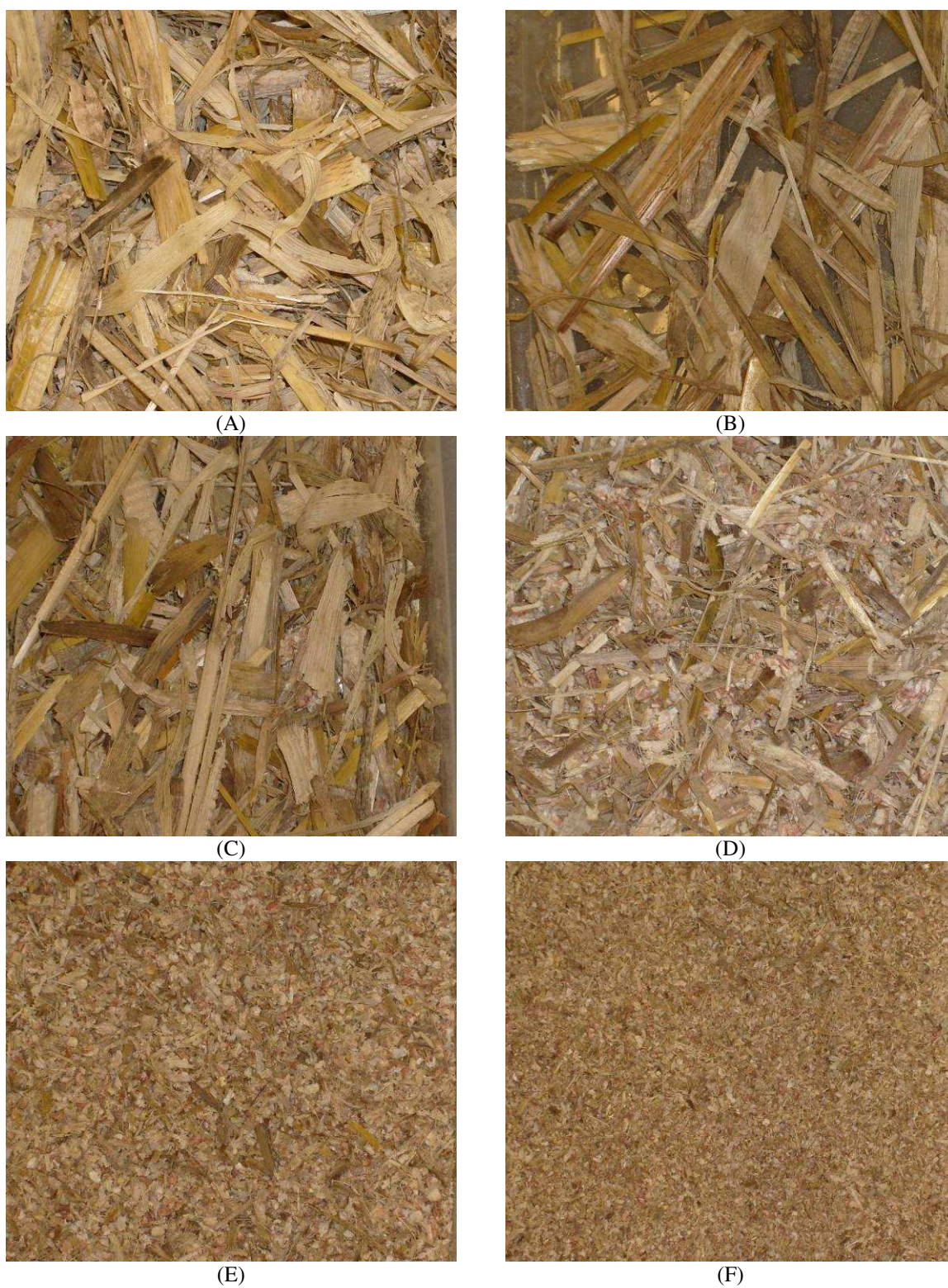
Figure A4. Photographs of stover material after particle reduction with a roller mill at a nominal feedrate of 84 kg/hr and roller gap setting of 0.0889 cm. Material collected over 5.08 cm screen (A), 2.54 cm screen (B), 1.27 cm screen (C), 0.635 cm screen (D), 0.318 cm screen (E) and above pan (F), are shown.
