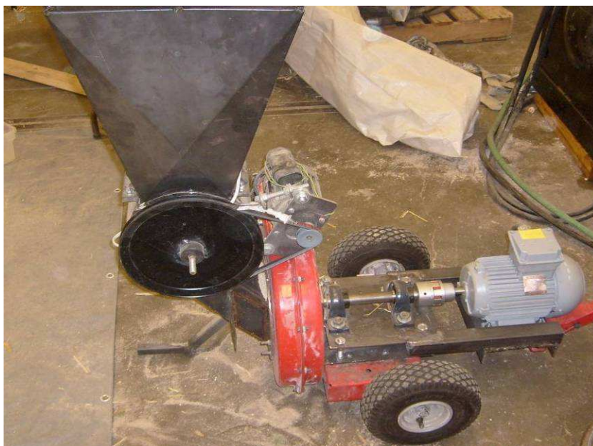
Figure 4. Hammermill showing motor drive and feed system attached.
