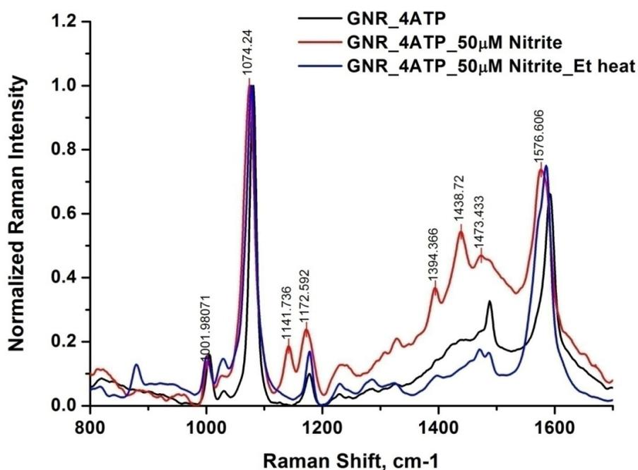
**Fig. 4** Raman spectra of 4ATP modified GNR (black), GNR-4ATP reacted with nitrite (red) and heated at 95°C (blue) in 20% ethanol.
