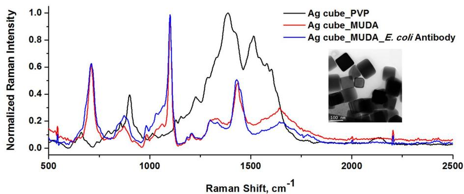
**Fig. 13** SERS spectra of silver nanocubes covered with PVP (black), MUDA (red) and MUDA and anti-*E. coli* antibody (blue). TEM image is silver nanocubes modified by MUDA and anti-*E. coli* antibody.
