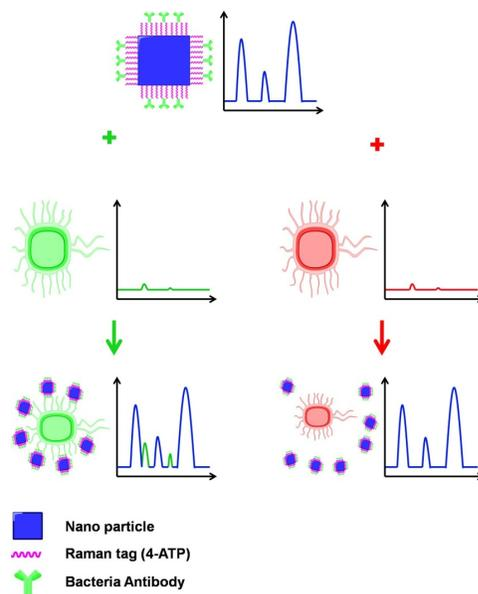
**Fig. 11** Scheme of dual recognition bacterial detection SERS nano probe
