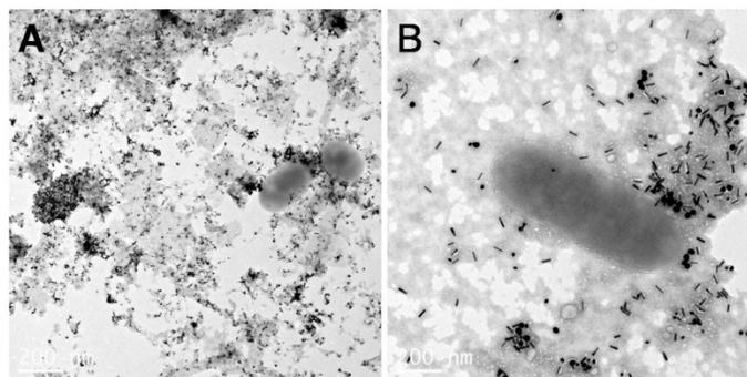
**Fig. 14** TEM image of gold nano probe with anti-*E. coli* antibody incubated with (A) *E. coli* and (B) *L. monocytogenes*.
