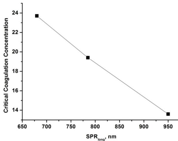
**Fig. 8** CCC of GNR-4ATP with different aspect ratios as a function of  $\text{SPR}_{\text{long}}$  band
