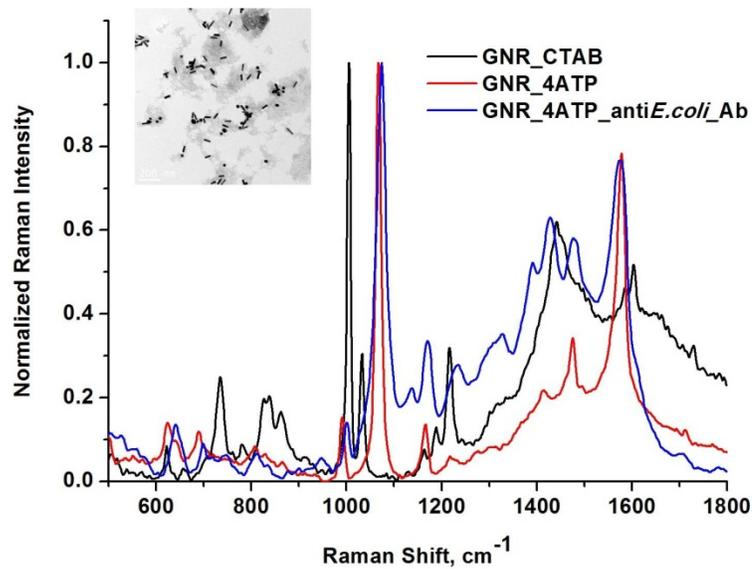
**Fig. 12** SERS spectra of gold nanorods covered with CTAB (black), 4-ATP (red) and 4-ATP and anti-*E. coli* antibody (blue). TEM image is GNRs modified by 4ATP and anti-*E. coli* antibody.
