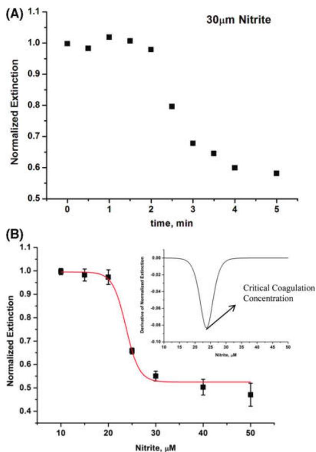
**Fig. 6** (A) Extinction of GNR-4ATP at wavelength of its  $\text{SPR}_{\text{long}}$  band, 785 nm, reacted with 30  $\mu\text{M}$  nitrite, as a function of incubation time at 95 °C. (B) Extinction of GNR-4ATP at wavelength of its  $\text{SPR}_{\text{long}}$  band, 680 nm, after 5 min incubation at 95 °C as a function of nitrite concentration.
