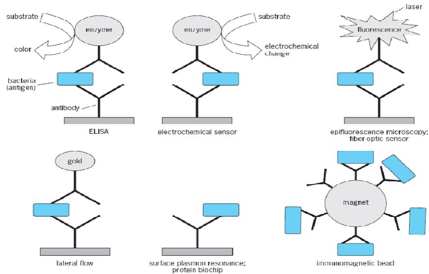
**Fig. 2** Various antibody-based detection schemes for pathogens (Bhunia and Lathrop 2003)
