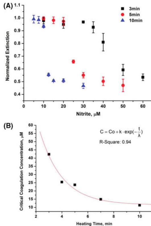
**Fig. 7** (A) GNR, with  $\text{SPR}_{\text{long}}$  at 680nm, particle solution extinction at 680nm after heating at different nitrite concentration and different heating time (B) CCC of GNR-4ATP with  $\text{SPR}_{\text{long}}$  at 680 nm as a function of heating time
