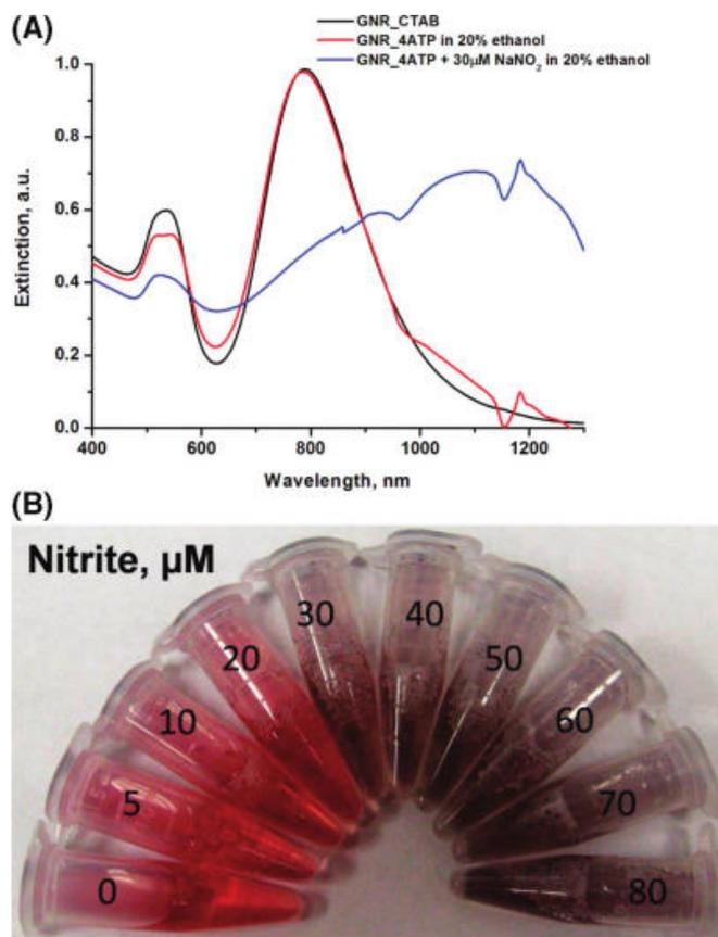
**Fig. 5** (A) Absorption spectra of CTAB covered GNR (black), GNR-4ATP in 20% ethanol solution (red), and aggregated GNR after heating in 20% ethanol (blue). (B) Photograph of GNR-4ATP reacted with various concentrations of nitrite after incubation in 20% ethanol at 95 °C
