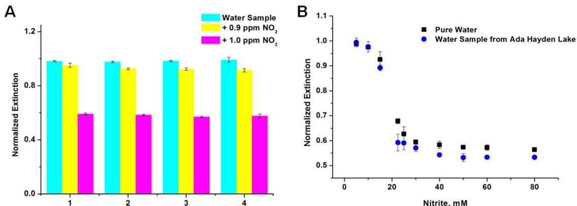
**Fig. 10** (A) Analysis of filtered water samples, 1. tap water of Ames 2. tap water of Iowa City 3. Nashua water monitoring well 4. Ada Hayden Lake; (B) Compare the test results between pure water and filtered water from Ada Hayden Lake.
