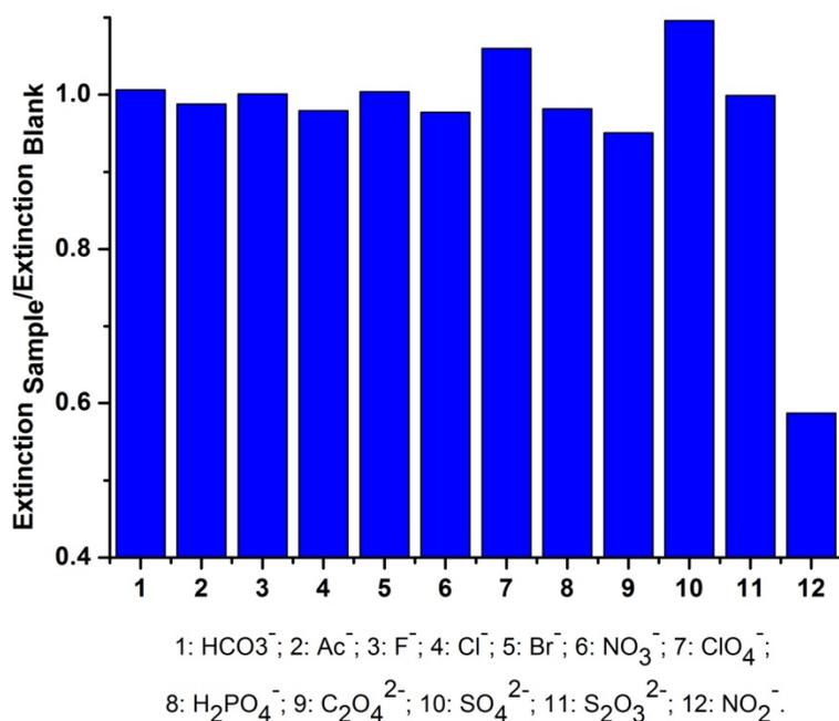
**Fig. 9** Selectivity of GNR nitrite sensor towards nitrite and other anions (The concentration of  $\text{SO}_4^{2-}$  and  $\text{S}_2\text{O}_3^{2-}$  were  $0.1 \text{ mM}$ , the concentration of  $\text{NO}_2^-$  was  $30 \mu\text{M}$  and the other anions concentration were  $1 \text{ mM}$ .)
