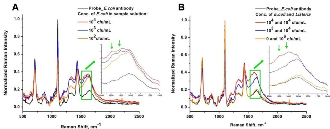
**Fig. 18** SERS spectra of silver nano probe covered with anti-*E. coli* antibody interacted with: (A) *E. coli* sample solution with different *E. coli* concentration; (B) *E. coli* and *Listeria* mixture sample solution.
