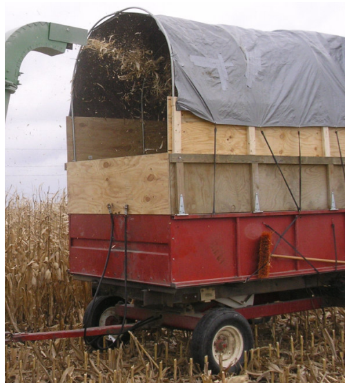
Figure 23: Instrumented stover wagon with integrated load cells used for stover collection
