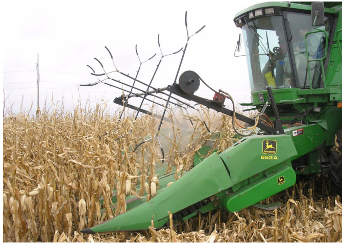
Figure 19: Corn reel in operation on 653A head during harvest
