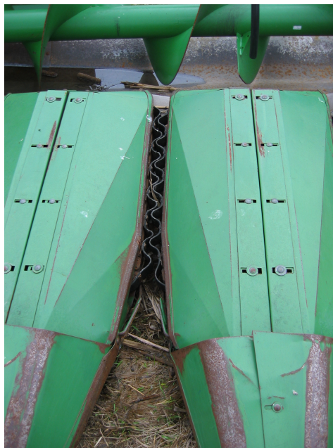
Figure 18: Gathering belts on 653A head used to control corn plant during harvest
