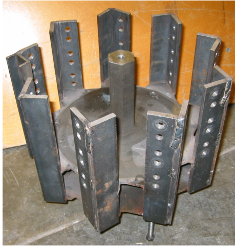
Figure 12: Jig for assembling double shear chopper sections
