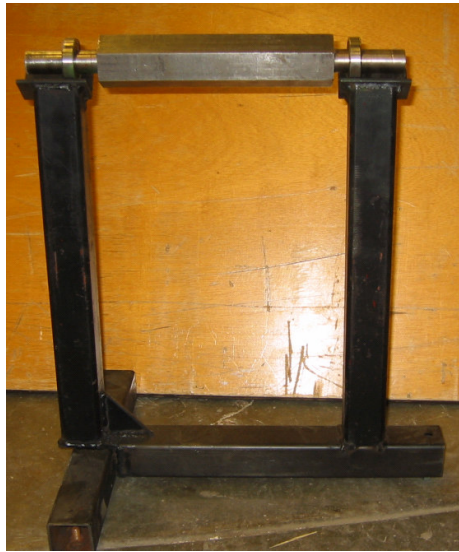
Figure 13: Balancing test stand for double shear chopper sections
