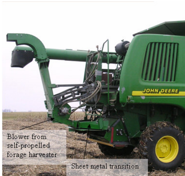
Figure 16: Image of forage blower and multi-function sheet metal transition
