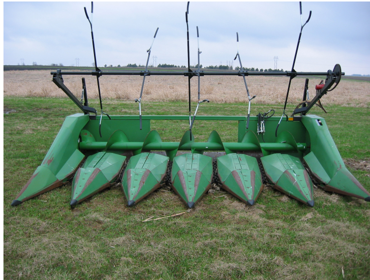
Figure 17: John Deere 653A row crop head with corn reel and modified auger tube section
