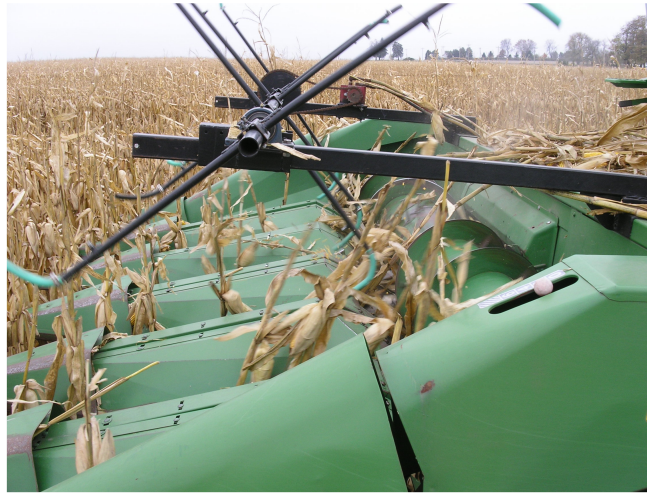
Figure 20: Original auger with 406 mm (16 in.) center tube and 102 mm (4in.) flighting in 653A head
