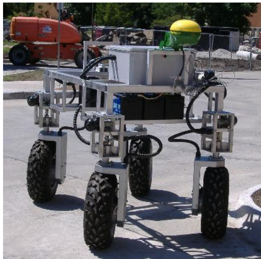
Figure 2.22: Crabbing steering mode
