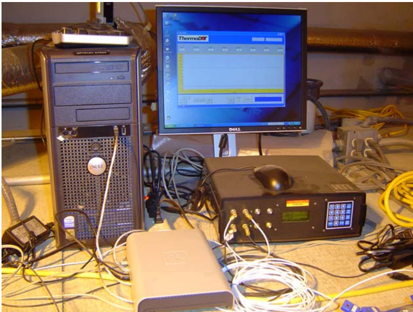
Figure 5.2: Core body temperature (CorTemp™) base unit and hosting PC.
