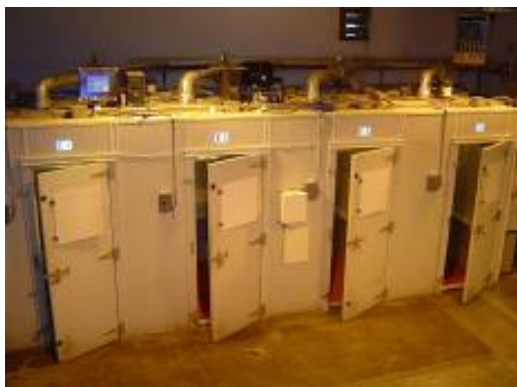
Figure 4.1: Environmentally controlled calorimeter chambers used in this study at the Iowa State University LEAP Laboratory
