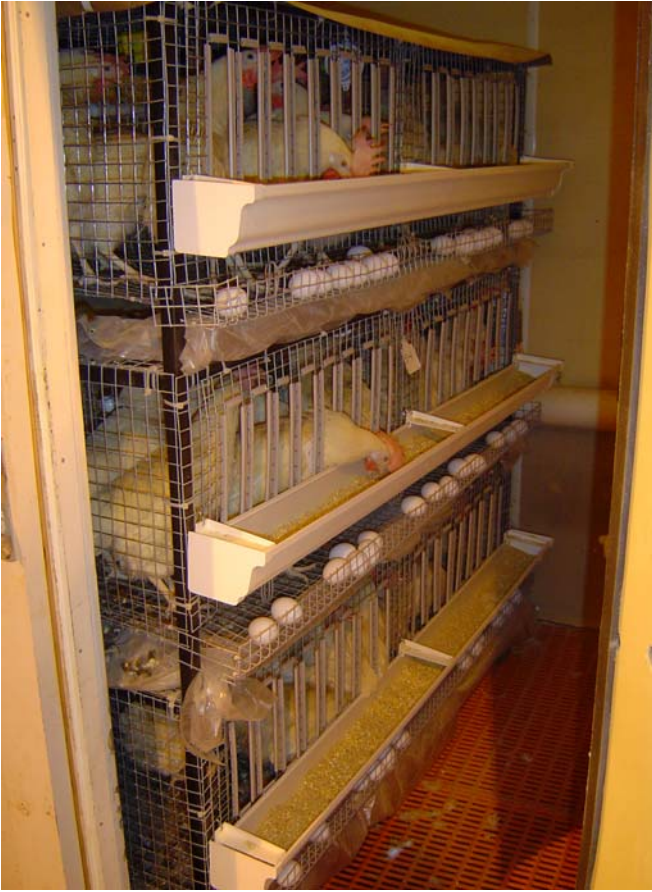
Figure 4.5: View of hen cages inside the calorimeter chamber during trial
