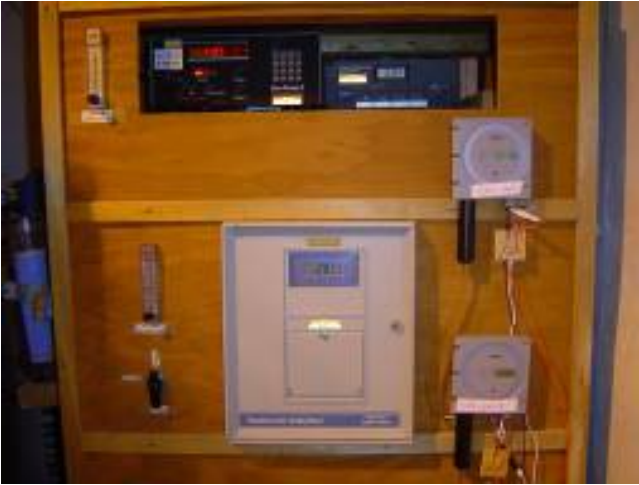
Figure 4.3: Gas and dew-point analyzers for measuring bioenergetic response of laying hens
