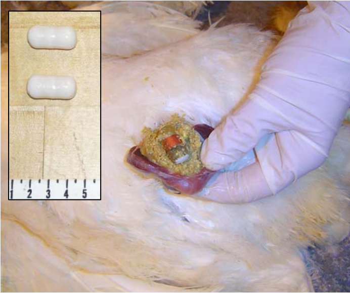
Figure 5.3: New core body temperature sensor (top left, cm scale) and recovery of used sensor.
