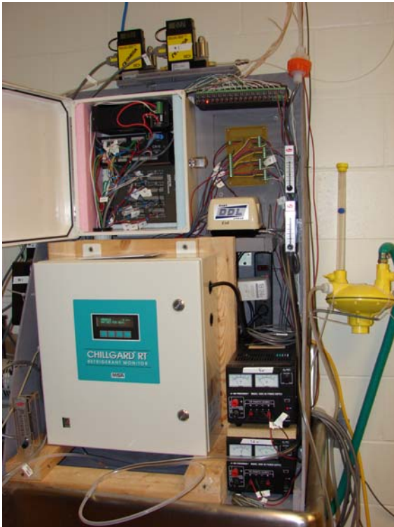
Figure 6.8: Instrumentation for control system
