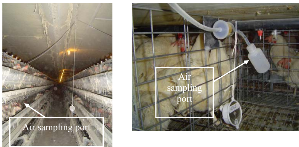
Figure 3.2: Photographical views of the bird-level sampling port in a caged house (sampling port placed inside an adjacent empty cage, T/RH logger inside cage and in aisle)
