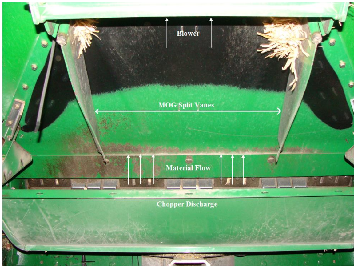
Figure 9: Transition from chopper to blower with MOG split vanes
