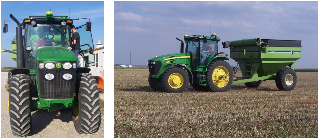
Fig. 7.2: An experimental system with a John Deere 7930 tractor and Alliance Product Group Parker grain cart. Two RTK GPS receivers were mounted on the tractor and two were mounted on the implement.
