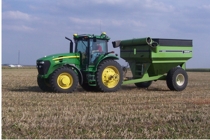
Fig. 5.2: An experimental system with a MFWD tractor (model 7930, Deere and Co., Moline, IL) and a single axle 500 bu (18 m 3 ) grain cart (model 500, Alliance Product Group, Kalida, OH). Two RTK GPS receivers were mounted on the tractor and two were mounted on the implement.
