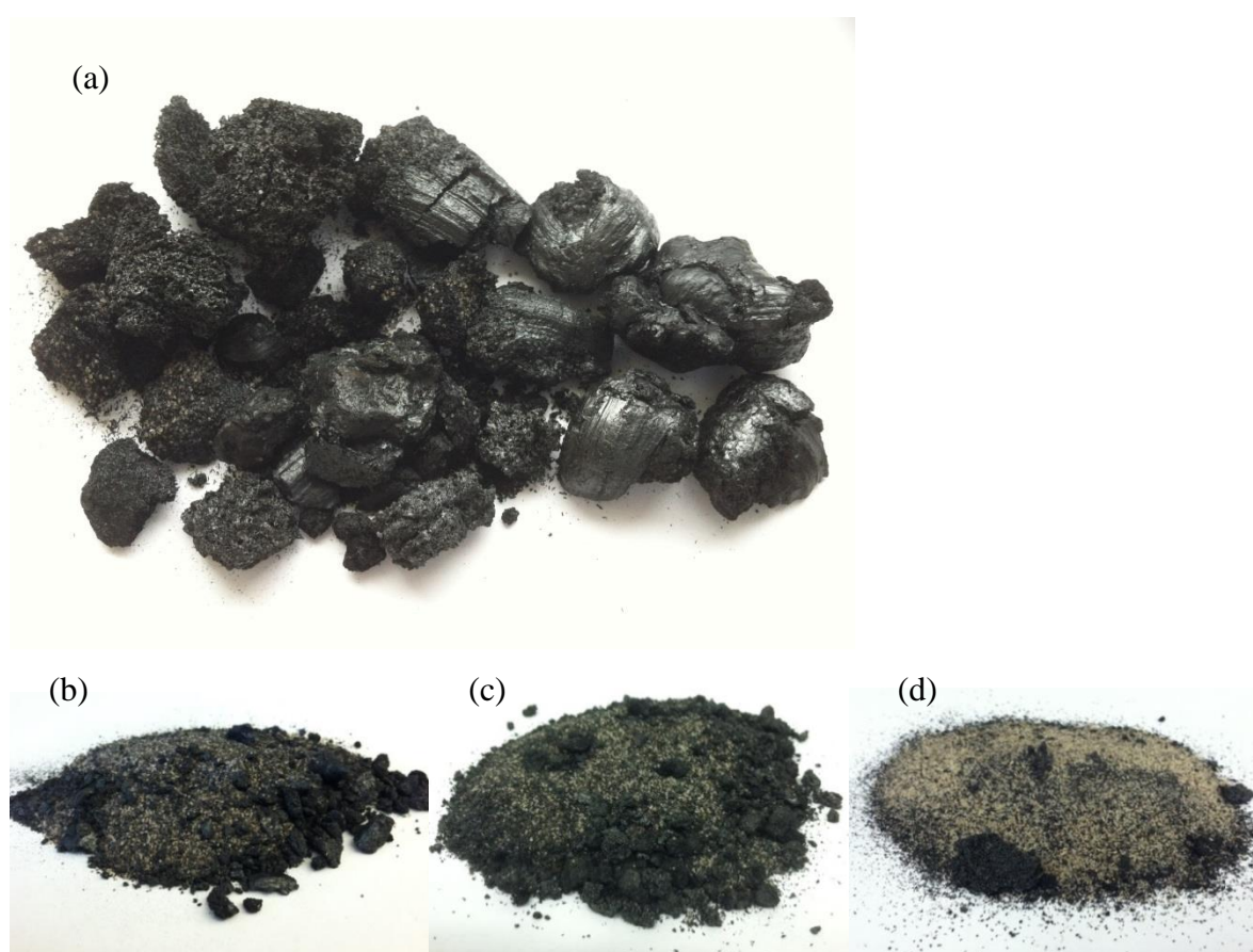
Figure 2. Char agglomerates and the fluidizing sand recovered from the fluidized bed pyrolyzer upon completion of (a) the control test (no oxygen admitted); (b) 2.1 vol% oxygen run; (c) 4.2 vol% oxygen run; (d) 8.4 vol% oxygen run
