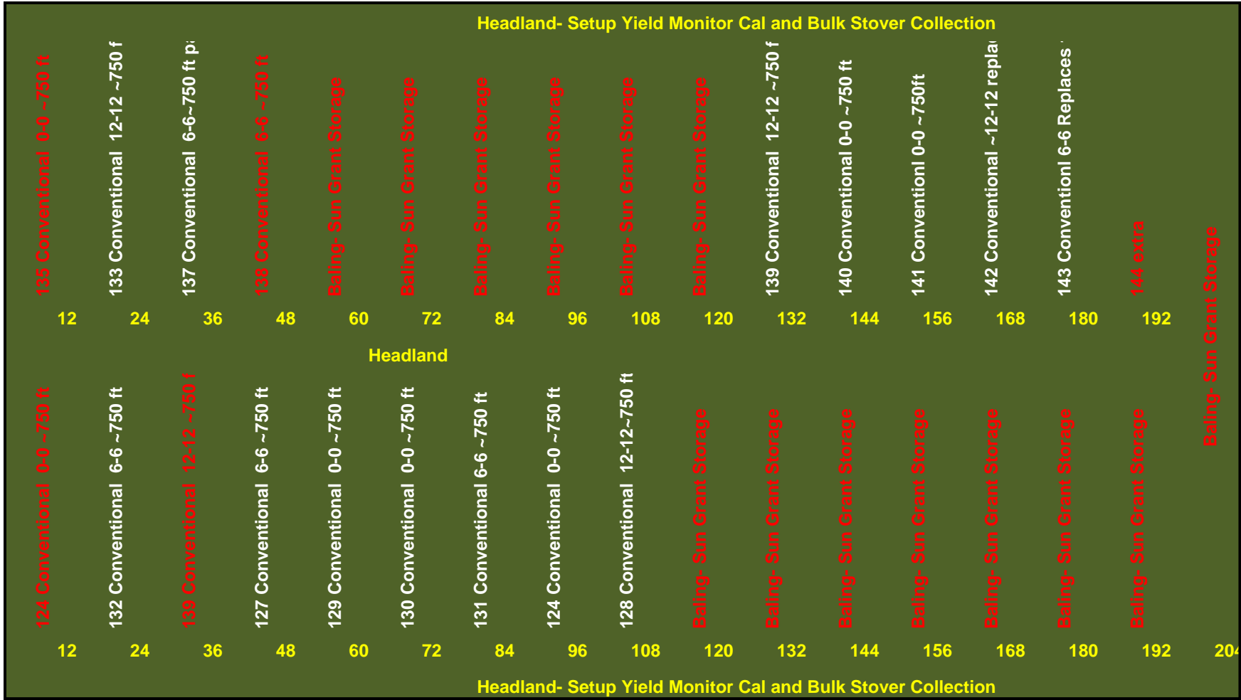
Figure 5-17: Separate layout of the higher-moisture grain field harvested for testing the combine. Each pass was laid out and assigned a number which is in the lower portion of the pass description was the running total of passes assigned throughout testing.
