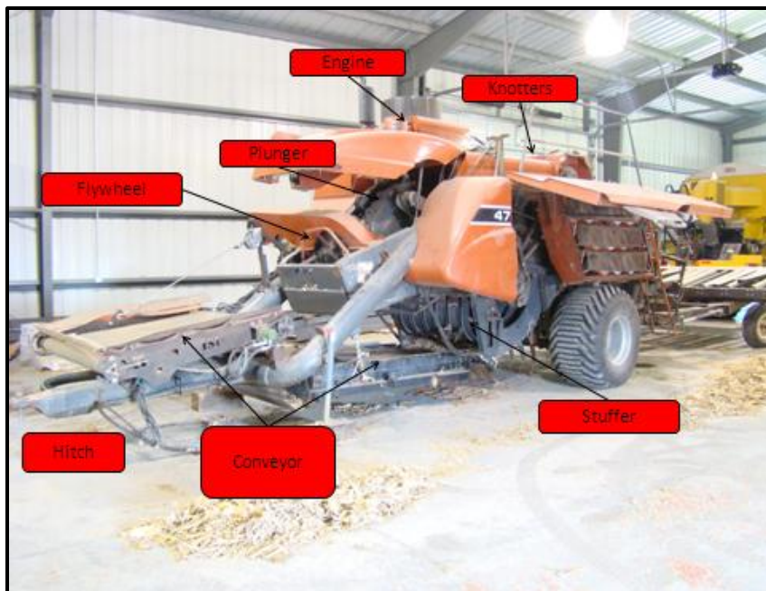
Figure 5-12: General layout of the components of the baler along with the modified components (conveyor and engine) for single-pass corn stover harvesting.
