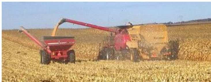
Figure 2-3: Vermeer Manufacturing's single-pass cob harvester system.
