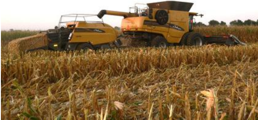
Figure 2-1: AGCO corporation's Challenger single-pass baler harvest system.
