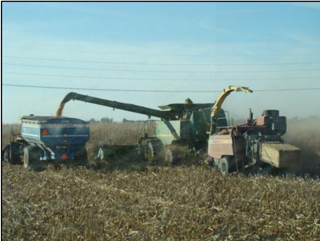
Figure 5-13: The John Deere 9860 with the AGCO 4790 single-pass baler harvesting grain and stover.
