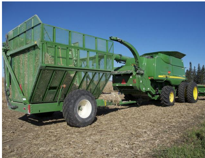
Figure 2-2: John Deere's and Hillco's single-pass cob harvester system developed in collaboration with Iowa State University.
