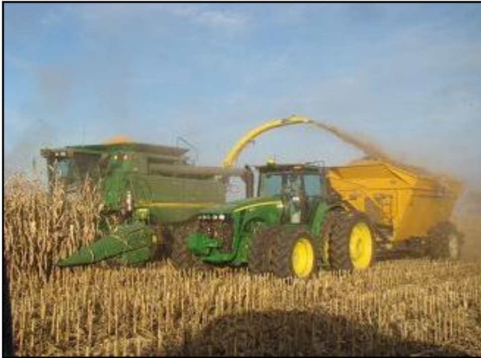
Figure 5-9: Combine in bulk stover collection configuration conveying stover into the Oxbo 1516 cart being towed by a John Deere tractor. This was one of the configurations tested.
