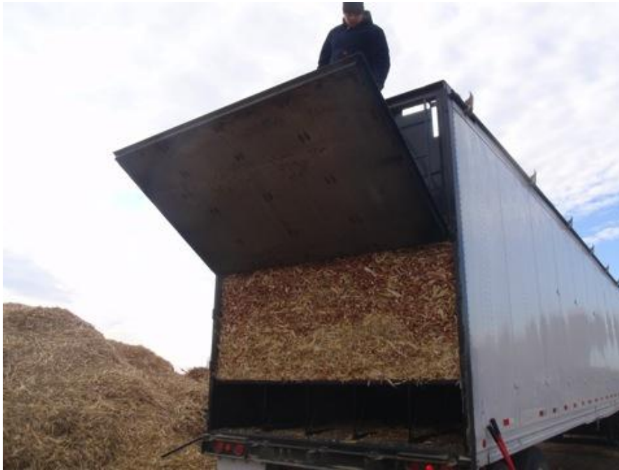
Figure 10. Low flowability of dried material.
