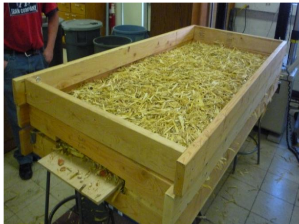
Figure 22. Place second and third frame
