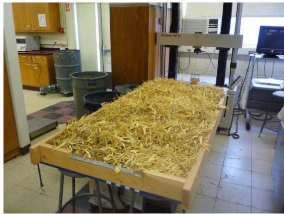
Figure 20. Fill test material up to frame level
