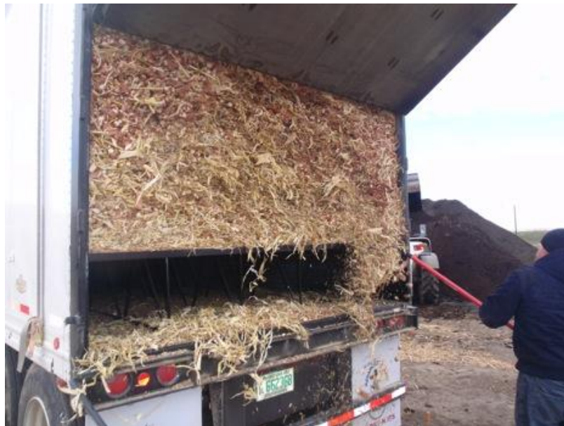
Figure 11. Laborious manual raking required to unload material.
