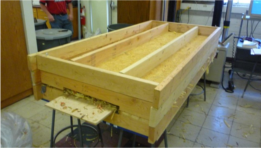
Figure 16. Scaled-up coefficient of friction test apparatus
