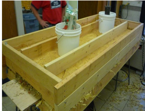
Figure 24. Place additional weights
