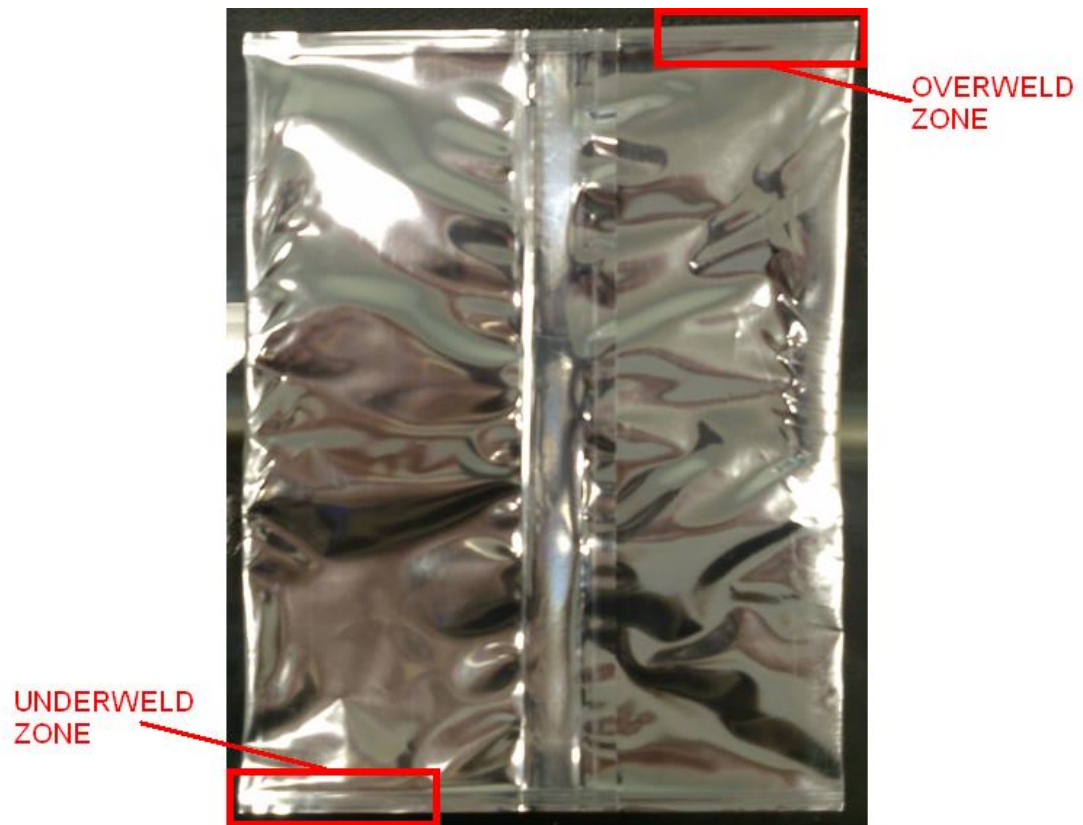
Figure 37 Locations prone to over weld and under weld
