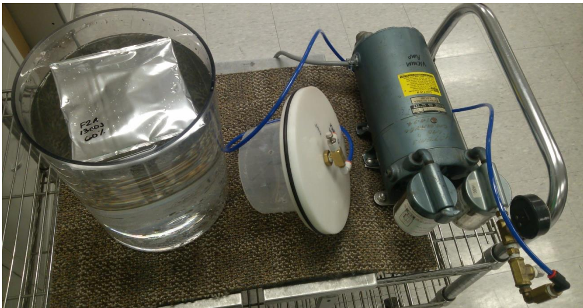
Figure 36 Vacuum chamber with specimen, lid, hose, and vacuum pump
