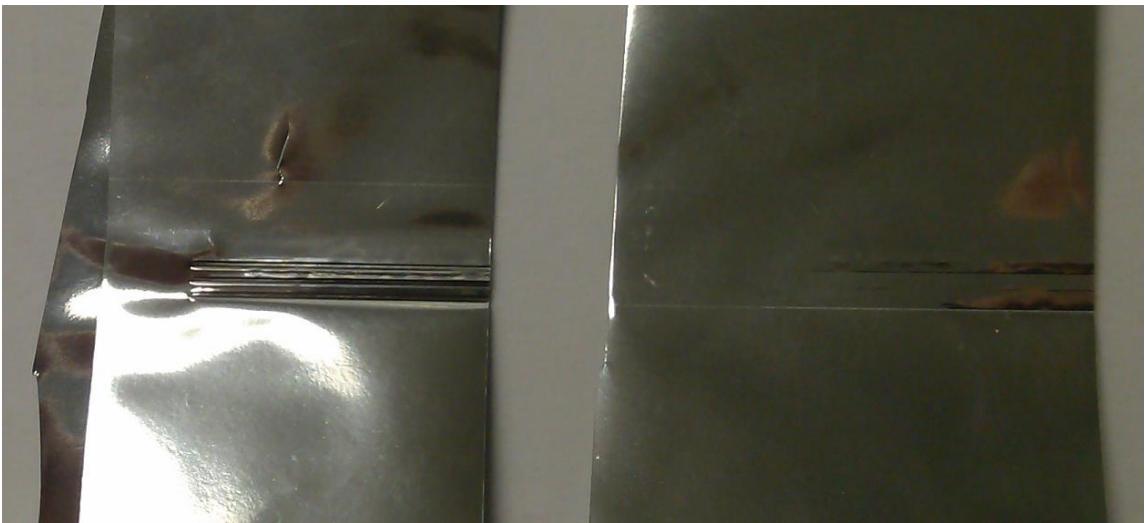
Figure 4 A complete weld (left) and example of under weld (right)
