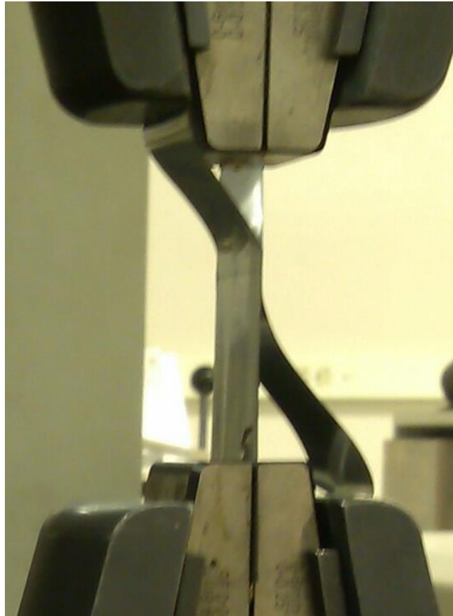
Figure 9 Photograph of specimen placement for shear strength testing
