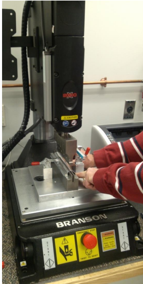
Figure 1 Branson 200X 30 kHz digitally controlled actuator
