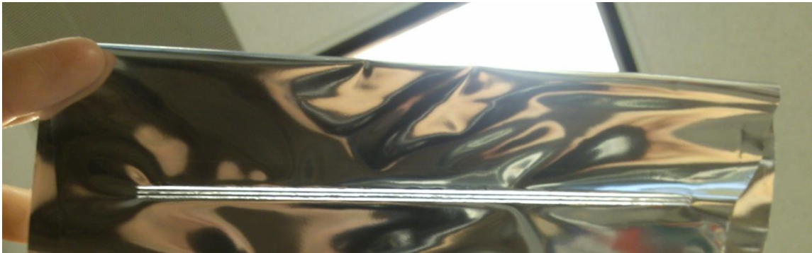
Figure 3 Excessive over weld condition
