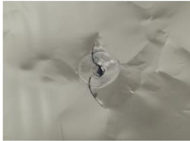
Figure 35 (Left) Burst test needle; (Right) Tear propagation at needle location
