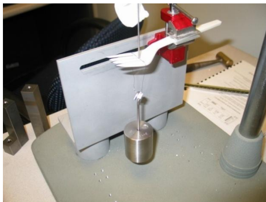
Figure 30. Step 8 fork layout (LVDT rod is touching the wire; wire is pulled flush against the utensil).
