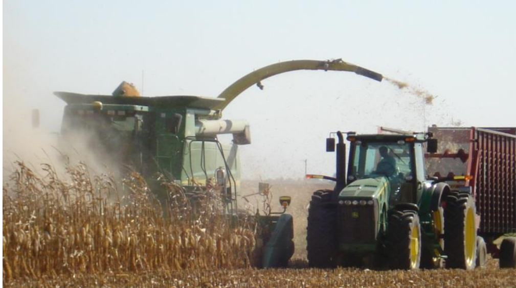
Figure 22: Modified 9860 STS combine for grain and corn stover collection.
