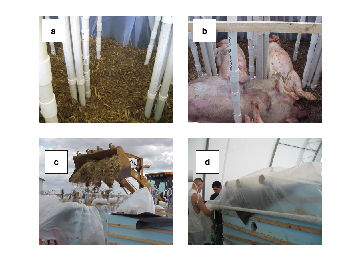
Figure 2. Inside view of test units and multi port gas-temperature sampling probe (a), (b), (c) and plastic sheet wraps (d)
