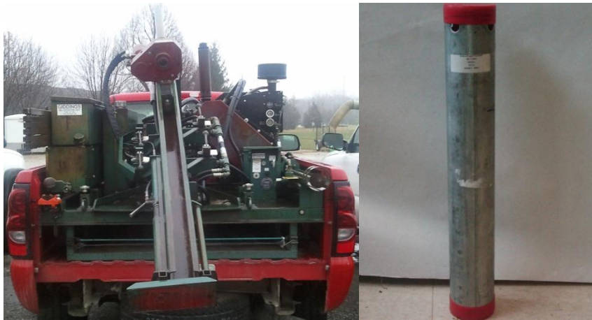
Figure 3.4 Soil sampling equipment Giddings Rig and Shelby tube used in the rig
