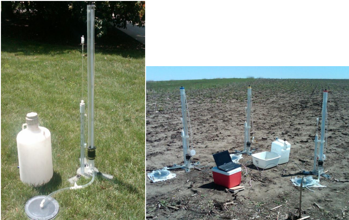
Figure 2.5 Tension Infiltrometer and equipment used
