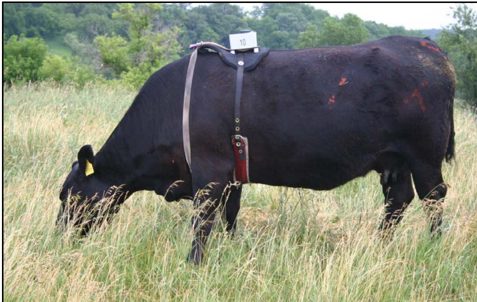
Figure 4: An Angus cow grazing in Bromegrass pasture fitted with a GPS HAWK unit.
