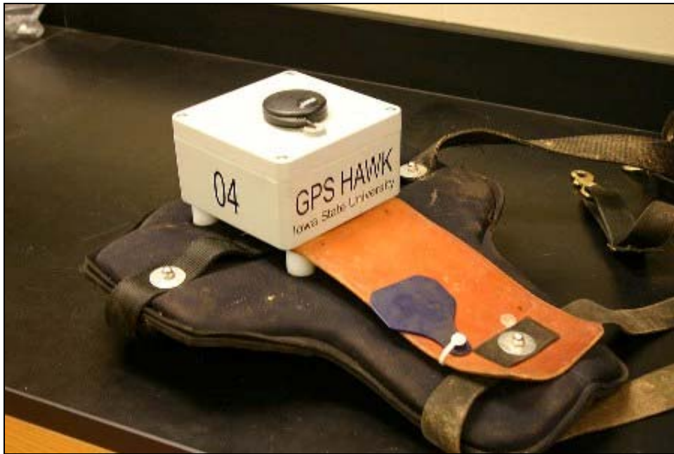
Figure 1: The GPS Herd Activity and Well-being Kit (HAWK) unit developed and used for the study.
