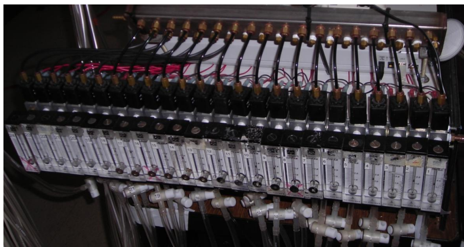
Figure 2: 24 port manifold, regulator valves and air gauges controlling individual sample's air flow.
