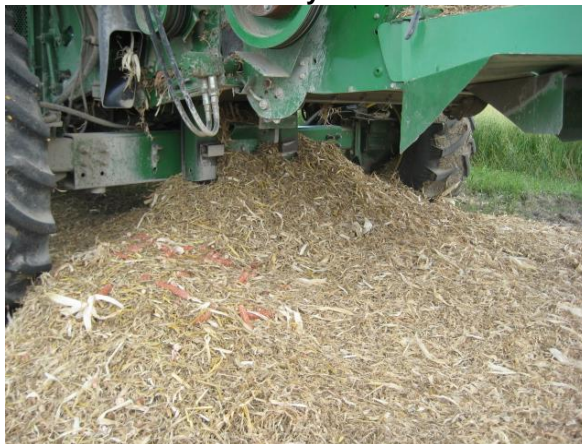
Figure 20. This figure shows that some cobs can still escape from the side air vents. This was taken after ten stationary tests.
