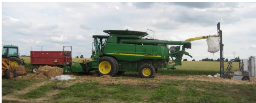
Figure 14. The stationary tests were conducted with combine and belt pick up head parked behind the barge box. A miniature bulk bag was located to collect all of the material exiting the spout.
