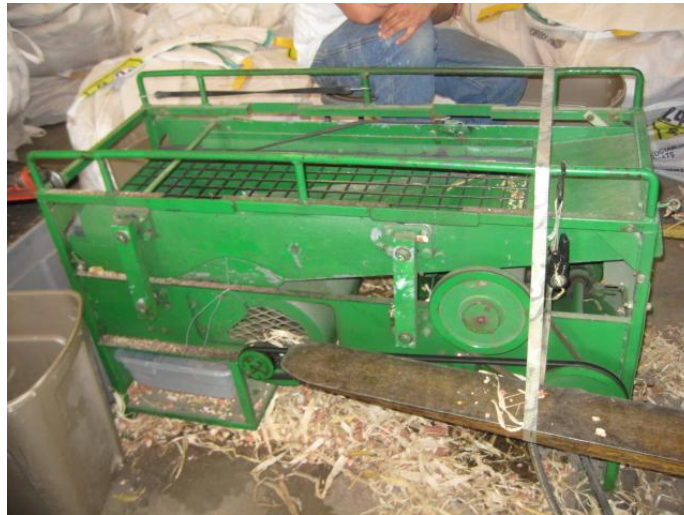
Figure 15. A shaker table was used to separate cobs from other material. A cob sieve was made with 50 mm openings which allowed cobs to pass through to the collection bin located underneath the table. A fan cleaned lighter material that fell through the sieve.
