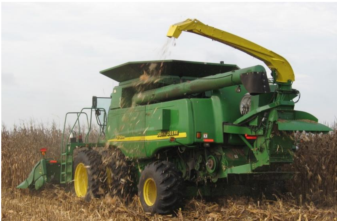
Figure 10. The cob separation system is active during this field test.
