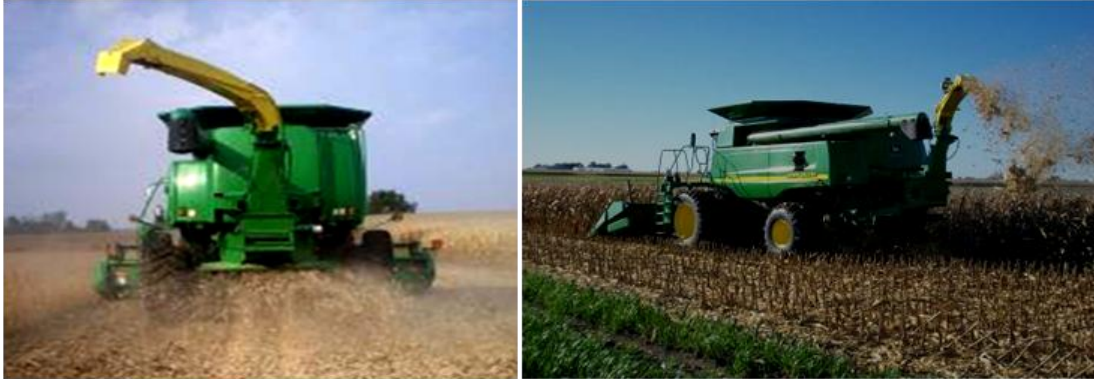
Figure 1. The stover attachment developed for a John Deere 9750 STS is shown in the spread mode while harvesting soybeans (left) and in collection mode while harvesting corn (right)
