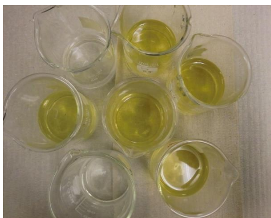
Figure 2. Filtrates from ozonated (yellow) and control (colorless) samples collected after 24 h soaking in Baermann funnels.
