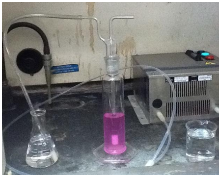
Figure 3. ozone generator, glass reactor and silicone tubing
