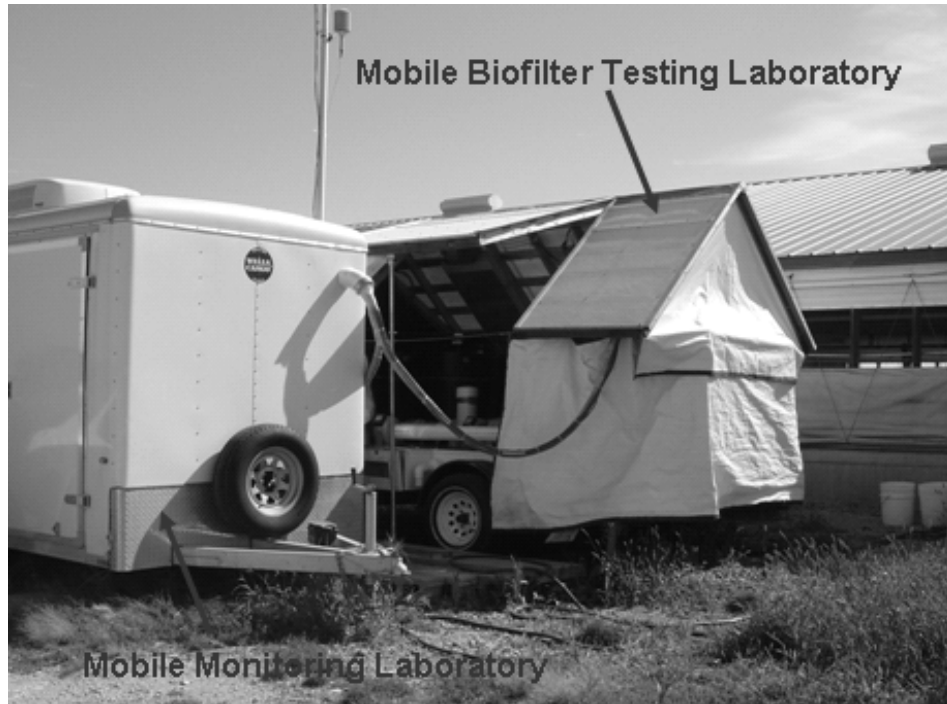
Figure 1a. Mobile pilot-scale biofilter laboratory and monitoring laboratory.
