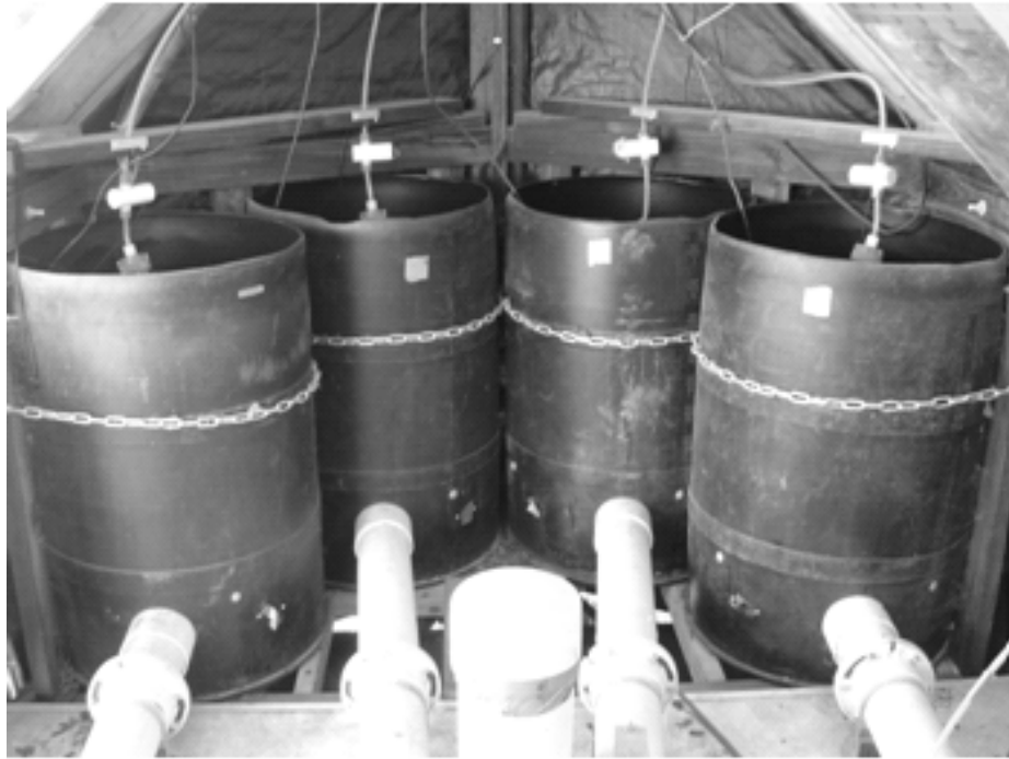
Figure 2a. Inside the biofilter testing laboratory showing four of eight reactor barrels.
