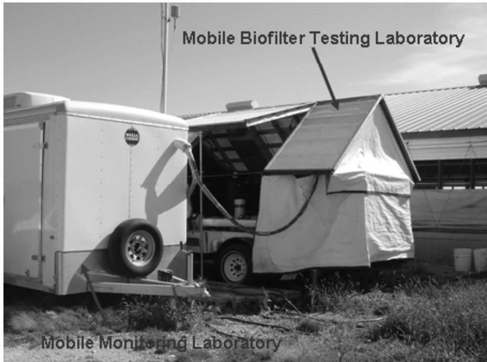
Figure 1a. Mobile biofilter testing laboratory and mobile monitoring laboratory.
