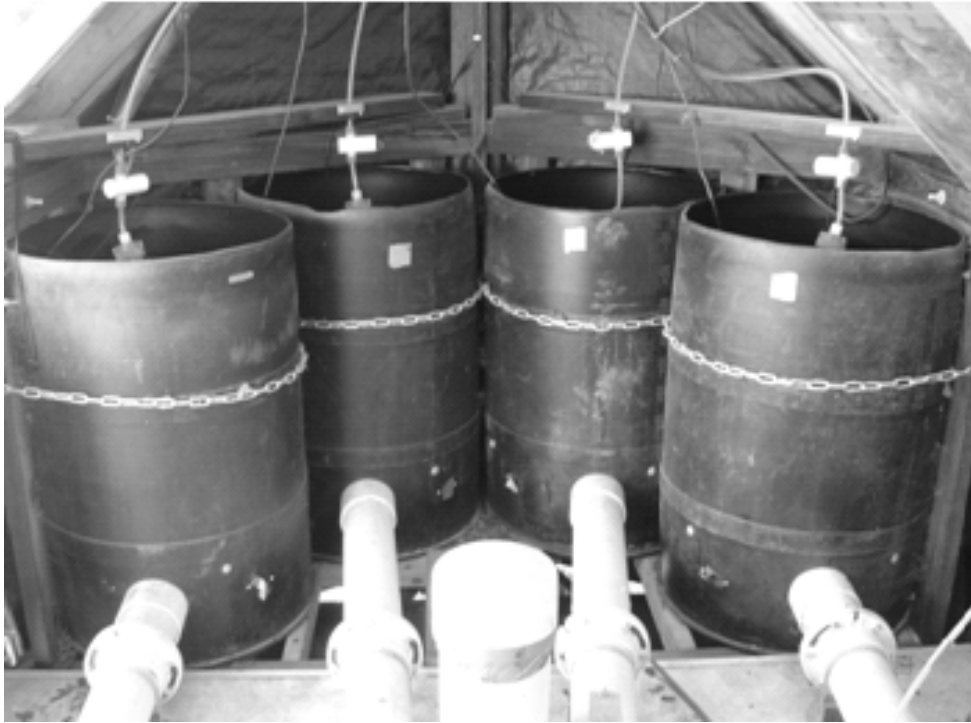
Figure 2a. Inside the biofilter testing laboratory showing four of eight total reactor barrels.
