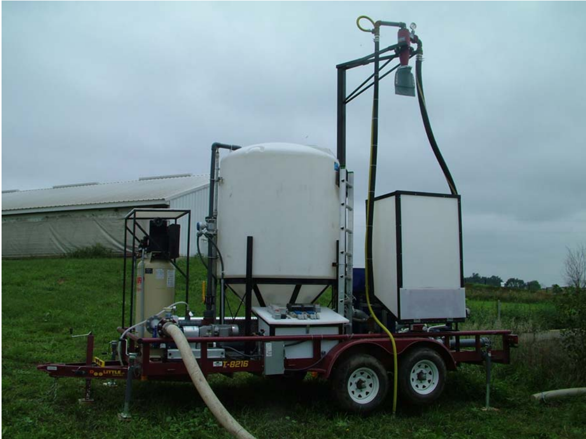
Figure 4.1. Palletized pilot-scale air sparged tank reactor with a hydrocyclone separator (ASTR-Hydrocyclone System)
