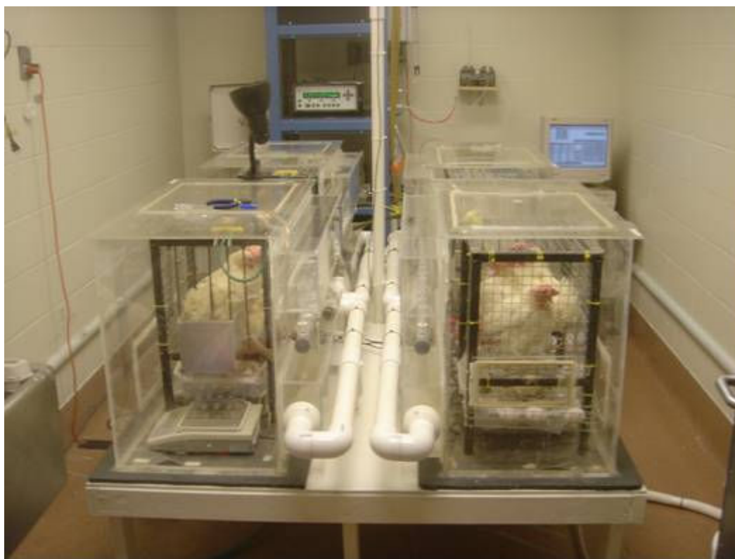
Figure 1a. An overview of the dynamic gas emissions chambers and measurement setup located in the Iowa State University Livestock Environment and Physiology (LEAP) Lab II.
