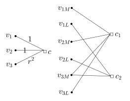
Figure 6.2: The left graph has edge labels from  $\mathbb{F}_4$ . The binary expanded graph on the right has check  $c_1$  of type T(3,1) and check  $c_2$  of type T(1,2), and is irregular since  $\alpha_1 + \beta_1 \neq \alpha_2 + \beta_2$ .
