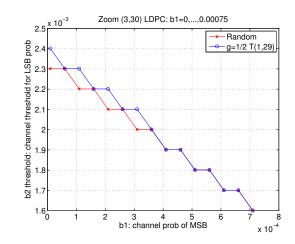
Figure 5.7: Thresholds for (3, 30)-regular codes, showing random vs. g = 1/2 and T(1, 29).
