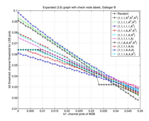
Figure 6.5: Thresholds of binary expanded graph codes obtained from (3, 6)-regular graphs under Gallager B decoding.
