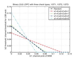
Figure 5.14: Three check types, with ratios  $g_1 = g_2 = g_3 = \frac{1}{3}$ .
