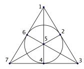
Figure 3.1: PG(2,2) with labels that correspond to the [7,4,3] Hamming code.
