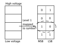
Figure 5.1: MLC flash cells and a binary mapping.
