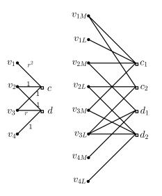
Figure 6.1: Nonbinary and binary expanded graph representations of a code over  $\mathbb{F}_4$
