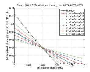
Figure 5.16: Three check types, with ratios  $g_1 = \frac{1}{2}, g_2 = \frac{1}{6}, g_3 = \frac{1}{3}$ .
