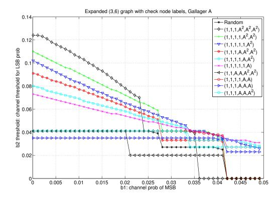
Figure 6.3: Thresholds of binary expanded graph codes obtained from (3, 6)-regular graphs using edge label sets from Table 6.1.
