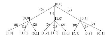
Figure 3.6: EG(1,3) WOM code, where the  $i^{th}$  layer of the tree corresponds to the  $i^{th}$  write.
