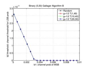
Figure 5.12: Thresholds for (5,50)-regular codes, Gallager A algorithm.
