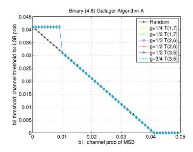
Figure 5.9: Thresholds for structured bit-interleaved (4, 8)-regular codes and corresponding random code.
