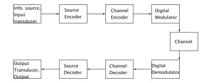
Figure 2.1: A model of a digital communication system [58].
