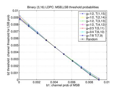
Figure 5.6: Thresholds for structured bit-interleaved (3, 16)-regular codes, showing the best of each  $\alpha_1 = 1, \ldots, 7$ .
