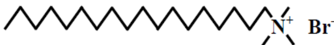
Figure 12. Chemical structure of octadecyltrimethylammonium (TMODA) bromide. TMODA is a long chain alkyl ammonium cation. It is reacted with Nafion to increase the hydrophobic regions of Nafion micellar pores, thus altering mass transport through the film and creating a structurally robust and protective microenvironment for cyanobacteria immobilization.
