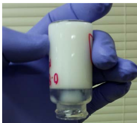
Figure 5.1 Photo of insoluble amorphous aluminum hydroxide precipitate upon hydrolysis of \text{Al}^{3+} , forming a semi-solid with a relatively unknown structure.
