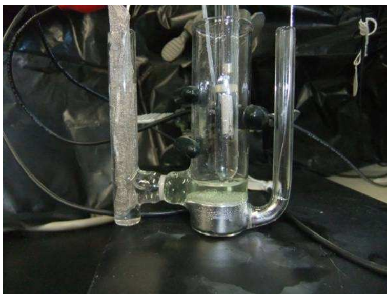
Figure 6.3: Picture of actual H-cell employed for bulk electrolysis reactions. Two chambers are separated by a medium porosity fritted-glass. The chamber on the left has a Pt mesh CE submerged in a stock electrolyte solution. The chamber on the right has a pool of Hg as the WE with a Pt wire electrical contact (far right). The Hg pool is covered with a solution of analyte and a calomel RE is dipped into the analyte solution. A Teflon hose supplying inert gas was used to blanket the reaction in order to prevent oxidation by dioxygen and help concentrate the solution by evaporation of the solvent and to help alleviate some \text{O}_{2(g)} .
