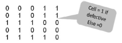
Figure 4.9. 2D representation showing defect filled cells as 1s, and defect-free cells as 0s
